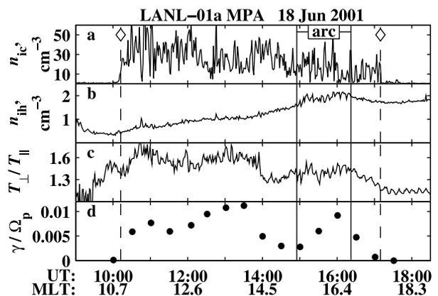
**Figure 2.** In situ measurements by the MPA instrument on LANL-01a. (a) Cold ion density. (b) Hot ion density. (c) Hot ion temperature anisotropy. (d) Dimensionless growth rate of the proton cyclotron instability calculated from linear Vlasov dispersion theory. The open diamonds correspond to the MLT locations indicated in Figure 1d and the detached proton arc was observed between the solid vertical lines.
