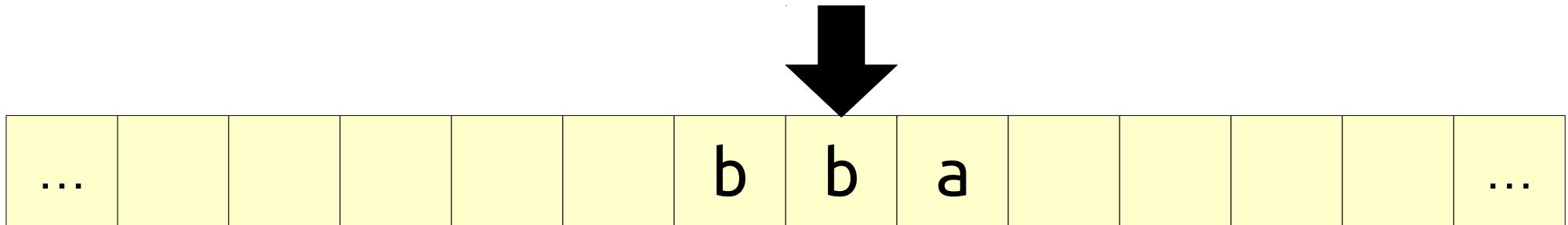
Although the tape ends with **bba** written on it, the original input string was **aab**. This shows that the TM accepts **aab**, not **bba**.
