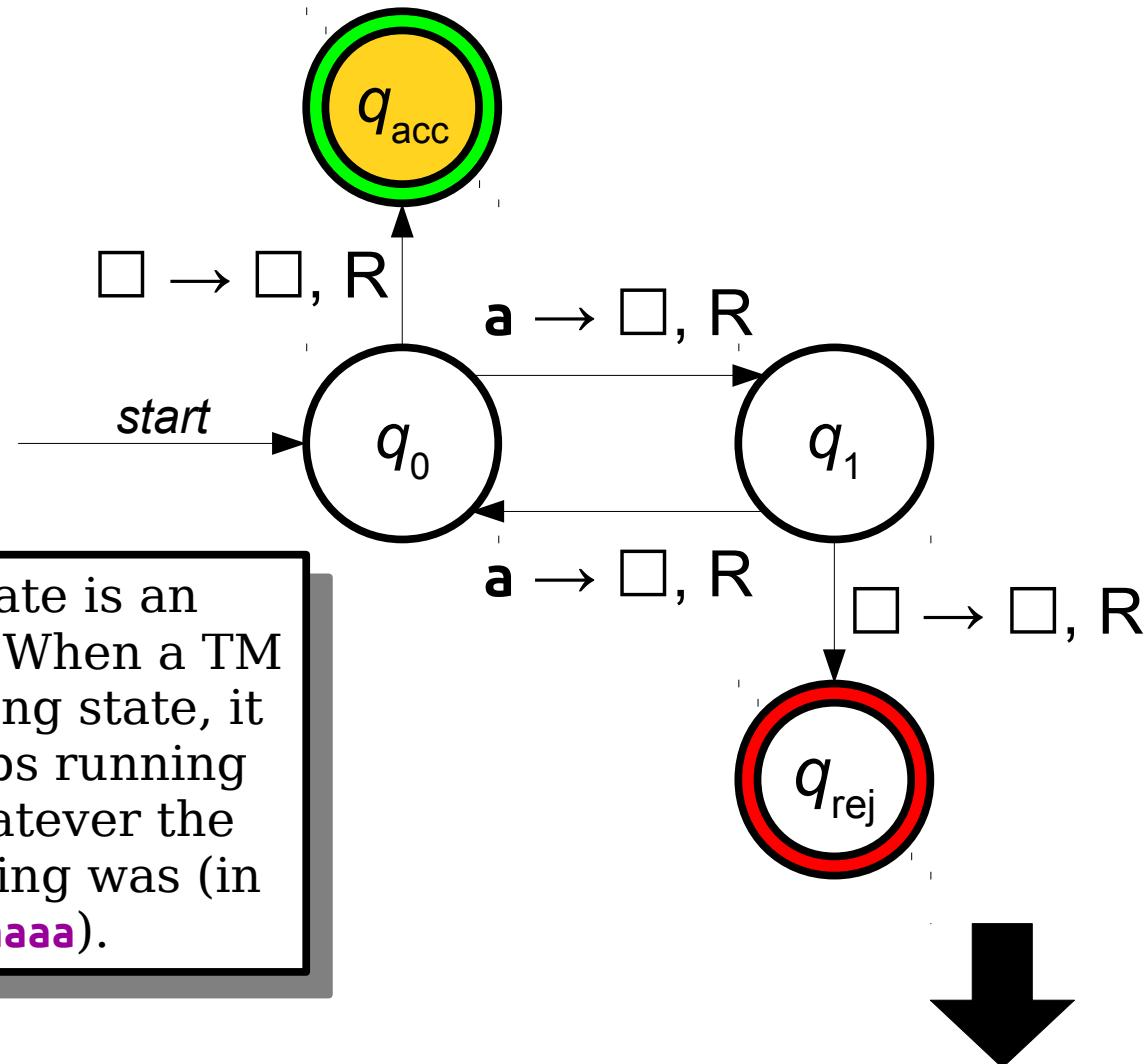
This special state is an **accepting state**. When a TM enters an accepting state, it *immediately* stops running and accepts whatever the original input string was (in this case, **aaaa**).
