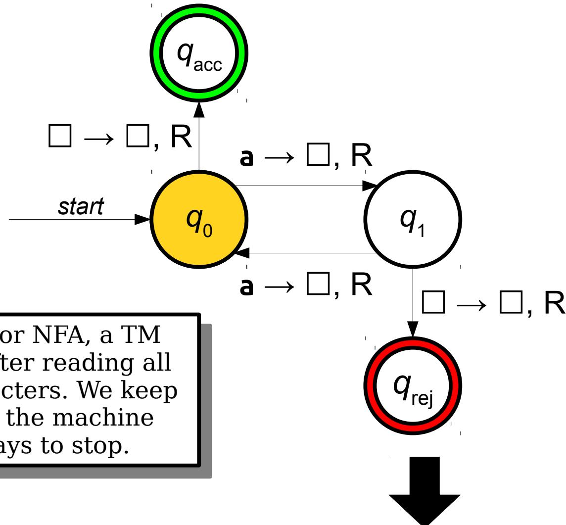
Unlike a DFA or NFA, a TM doesn't stop after reading all the input characters. We keep running until the machine explicitly says to stop.
