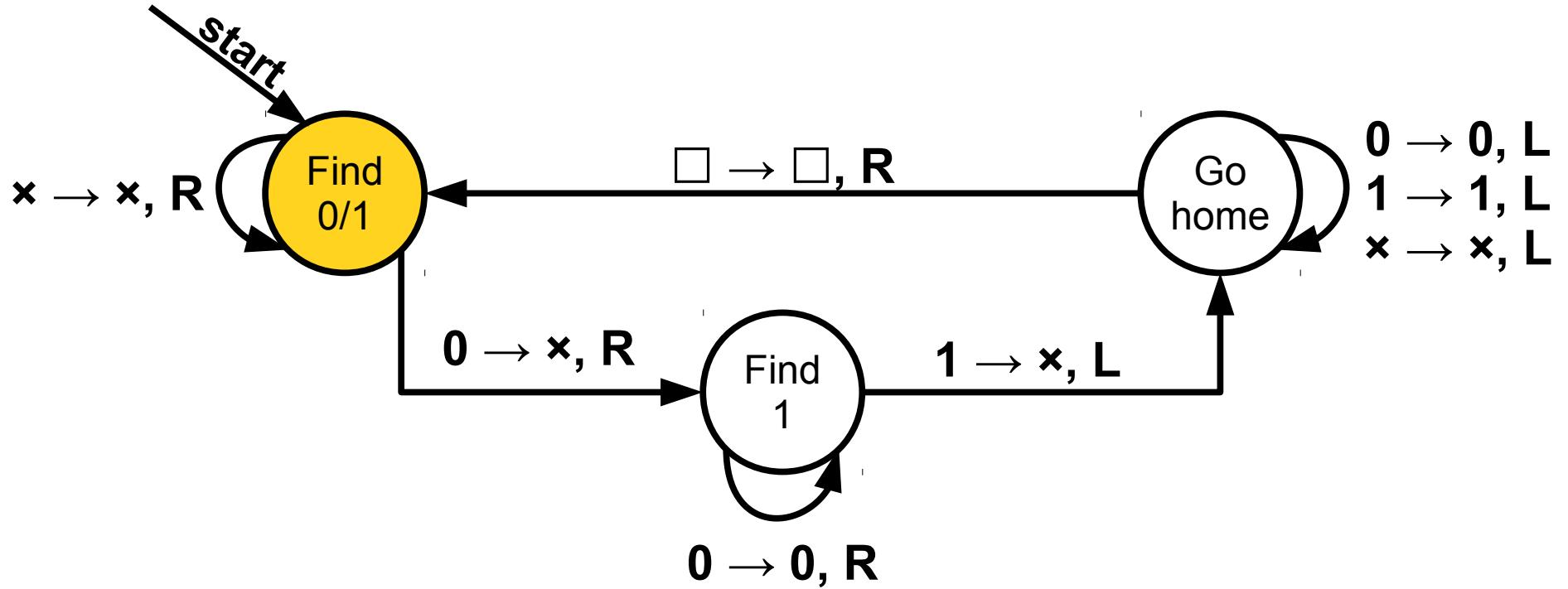
Diagram illustrating the computation step by step:
