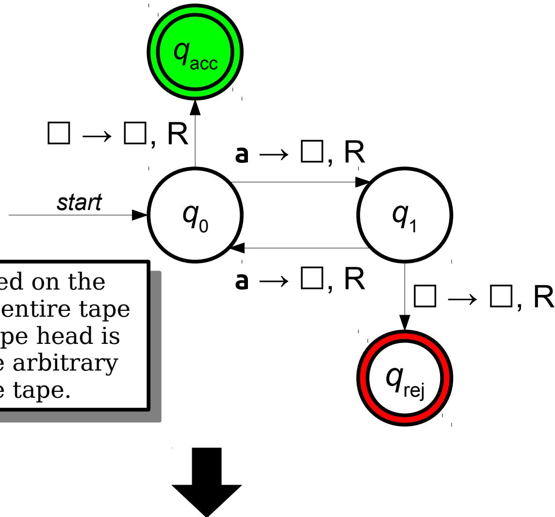
If the TM is started on the empty string  $\epsilon$ , the entire tape is blank and the tape head is positioned at some arbitrary location on the tape.
