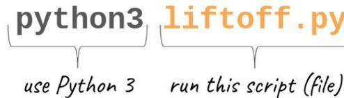
Figure 3: The command line command you would use to run your `liftoff.py` program.
