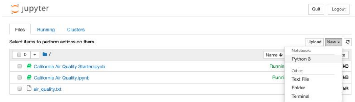
Figure 5: To create a new Python notebook, click on New > Python 3 at the top right of the browser tab that opens after you run jupyter notebook .
