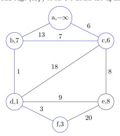
Finally node e is extracted and edge (c, e) is added to A. After this step the Fibonacci heap will be empty and Prim's Algorithm will return A.
