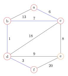
The next edge in the sorted order is (c, e). We union the sets containing c and e and add edge (c, e) to A. At this point all nodes are contained in the same set and so no further edges are added to A.
