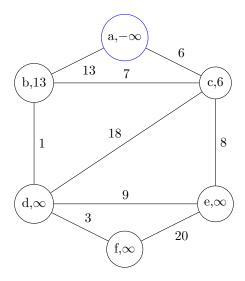
Since d(c) is now the smallest value in the Fibonacci heap, we visit node c. Because  $\pi(c) = a$  we add edge (a,c) to the set A. We then update the distance estimates and parent fields of nodes that have edges connecting to c. Thus we set d(b) = 7, d(d) = 18, d(e) = 8, and  $\pi(b) = c$ ,  $\pi(d) = c$ , and  $\pi(e) = c$ .
