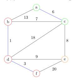
The next edge in the sorted order is (b,c). We union the sets containing b and c and add edge (b,c) to A.
