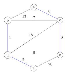
Following the merge operations the remaining supernodes are  $\{a, c, e\}$  and  $\{b, d, f\}$ . The superedge between these supernodes is defined by the real-edge (b, c). Thus we add edge (b, c) to the MST and following another merge operation we are left with only one supernode at which point the algorithm terminates.
