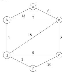
We begin by creating a new set for each node in the graph. We then being iterating over the edges in non decreasing order. The first edge we examine is (b, d). This edge connects nodes b and d which are currently not part of the same set. We thus include this edge in A and union the sets containing b and d.
