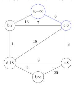
Node b is extracted next and we add edge (b,c) to A. We then set d(d)=1 and  $\pi(d)=b$ .
