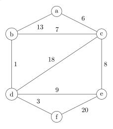
Suppose we select node a to be the source node, s. We then extract node a from the Fibonacci heap and set d(b) = 13, d(c) = 6 and  $\pi(b) = a$ ,  $\pi(c) = a$ .
