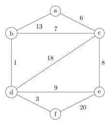
In the first iteration, we select the minimum superedge of each supernode. Since after initialization every node is a supernode and every edge is a superedge, this is equivalent to selecting the minimum weighted edge of each node.
