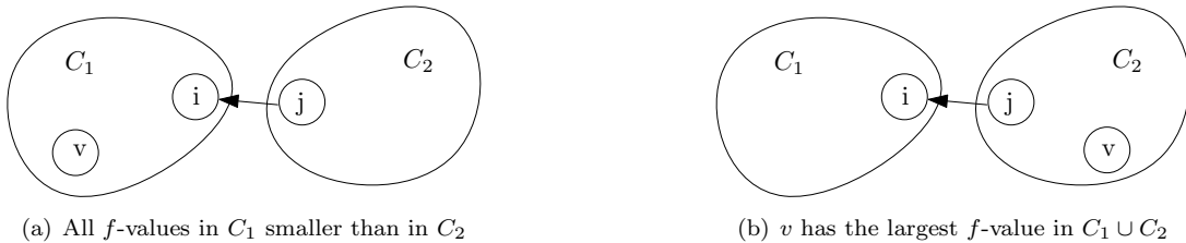
Figure 7: Proof of Key Lemma. Vertex v is the first in C_1 \cup C_2 visited during the execution of DFS-LOOP on G^{rev} .
