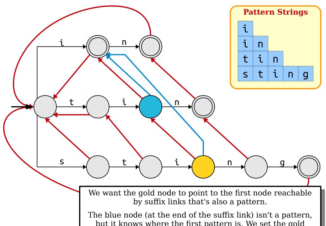
but it knows where the first pattern is. We set the gold node's output link to equal the blue node's output link.
