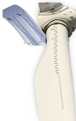
Vortex generators concentrate flow (1-2% AEP Improvement)
