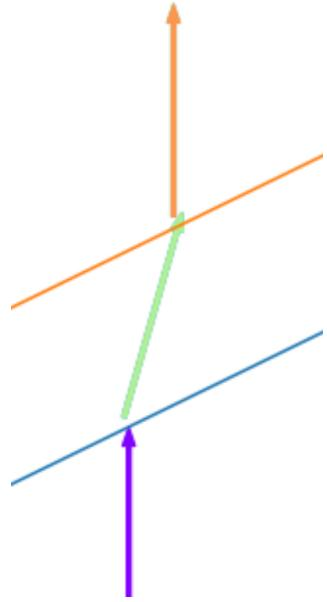
1. First, you need to compute the index of refraction (IOR) ratio:  $\frac{n_1}{n_2}$ . The tricky part here is that  $n_1$  and  $n_2$  change depending on where the ray starts.  $n_1$  is always the IOR of the medium in which the ray starts for the transmission.  $n_2$  is always the IOR of the medium in which the ray ends up for the transmission.
