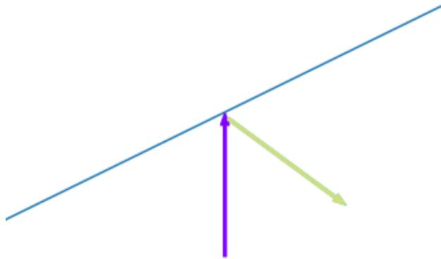
Suppose our ray is initially traced as the purple ray and intersects the blue edge of a reflective object. The ray gets reflected by the object to then continue in a different direction from which it began. In code, we represent the reflected ray as an entirely new ray object. This new reflected ray is represented by the light-green ray in the diagram pointing to the lower-right.
