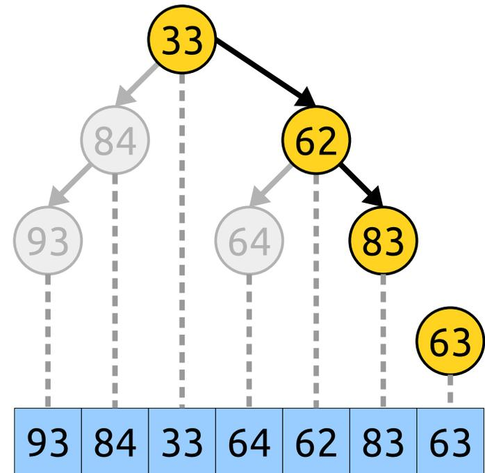
**Observation 1:** After adding this node, it must be the rightmost node in the tree. (An inorder traversal of a Cartesian tree gives back the original array.)
