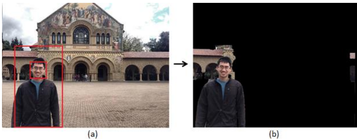
Figure 7: (a) Mask determined by bounding boxes fed into GrabCut to produce (b).
