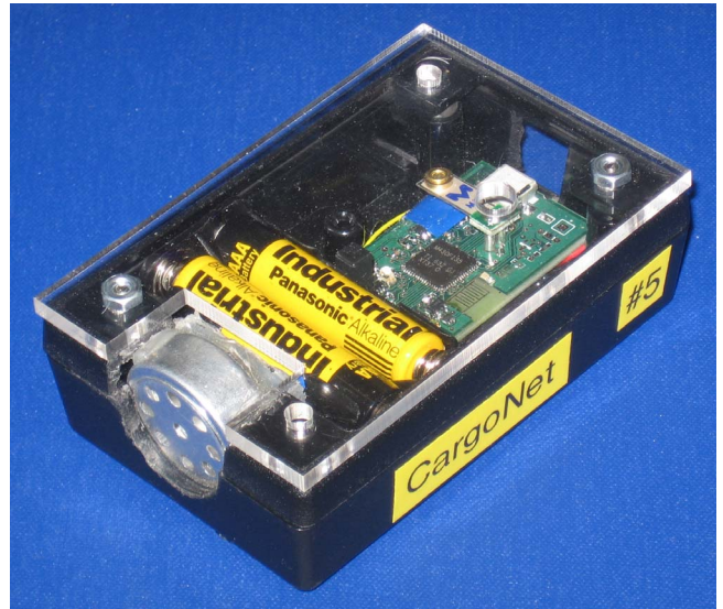
Figure 5. A packaged prototype CargoNet tag used in tests, showing the piezoelectric microphone that can wake the microcontroller on loud sounds.
