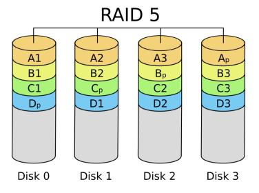
Striping + 1 parity disk: adds performance and reliability at lower storage cost
