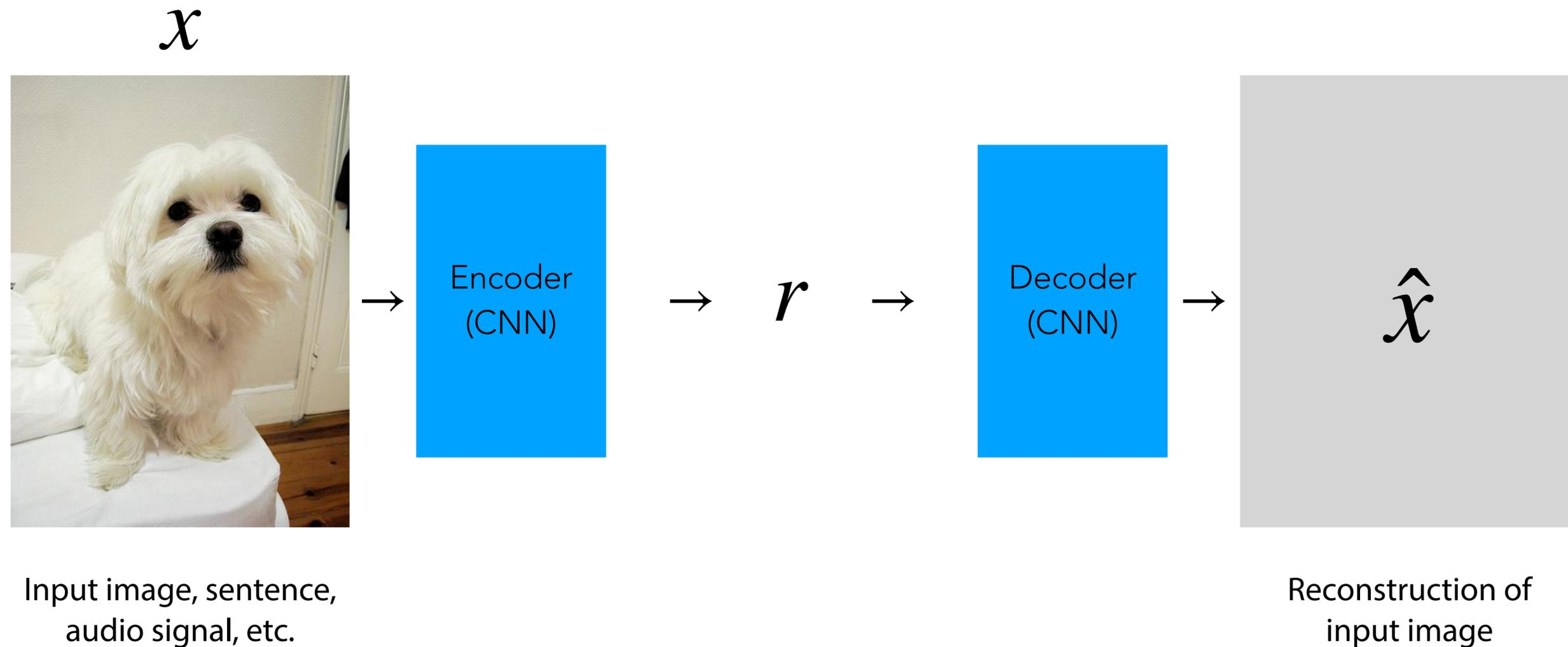
If the encoder is producing a "good" representation, a reasonably-sized decoder should be able to produce **reconstruction**  $\hat{x}$  very close to **input**  $x$  from **representation**  $r$
