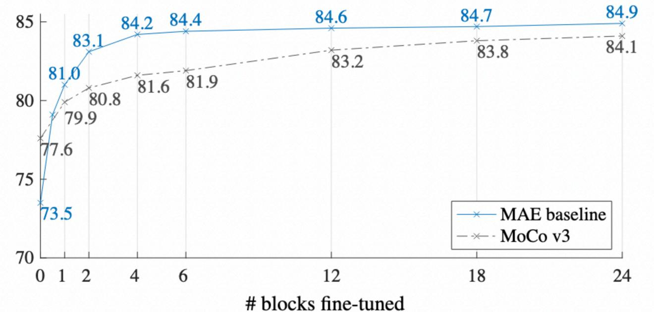
Figure 9. **Partial fine-tuning** results of ViT-L w.r.t. the number of fine-tuned Transformer blocks under the default settings from Table 1. Tuning 0 blocks is linear probing; 24 is full fine-tuning. Our MAE representations are less linearly separable, but are consistently better than MoCo v3 if one or more blocks are tuned.
