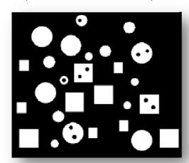
Write a pseudo-code description of an algorithm to count the number of widgets with holes and the number of widgets without holes. Include a simple block diagram of the algorithm to make it easy to understand. State any assumptions you make in your algorithm about the size or shape of the widgets.
