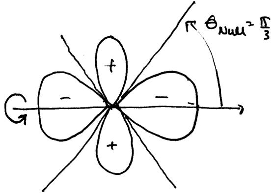
$$\begin{aligned} \text{Curve is } \cos\left(\frac{\pi d}{\lambda} \cos \theta\right) \Big|_{d=\lambda} \\ = 2 \cos(\pi \cos \theta) \end{aligned}$$
