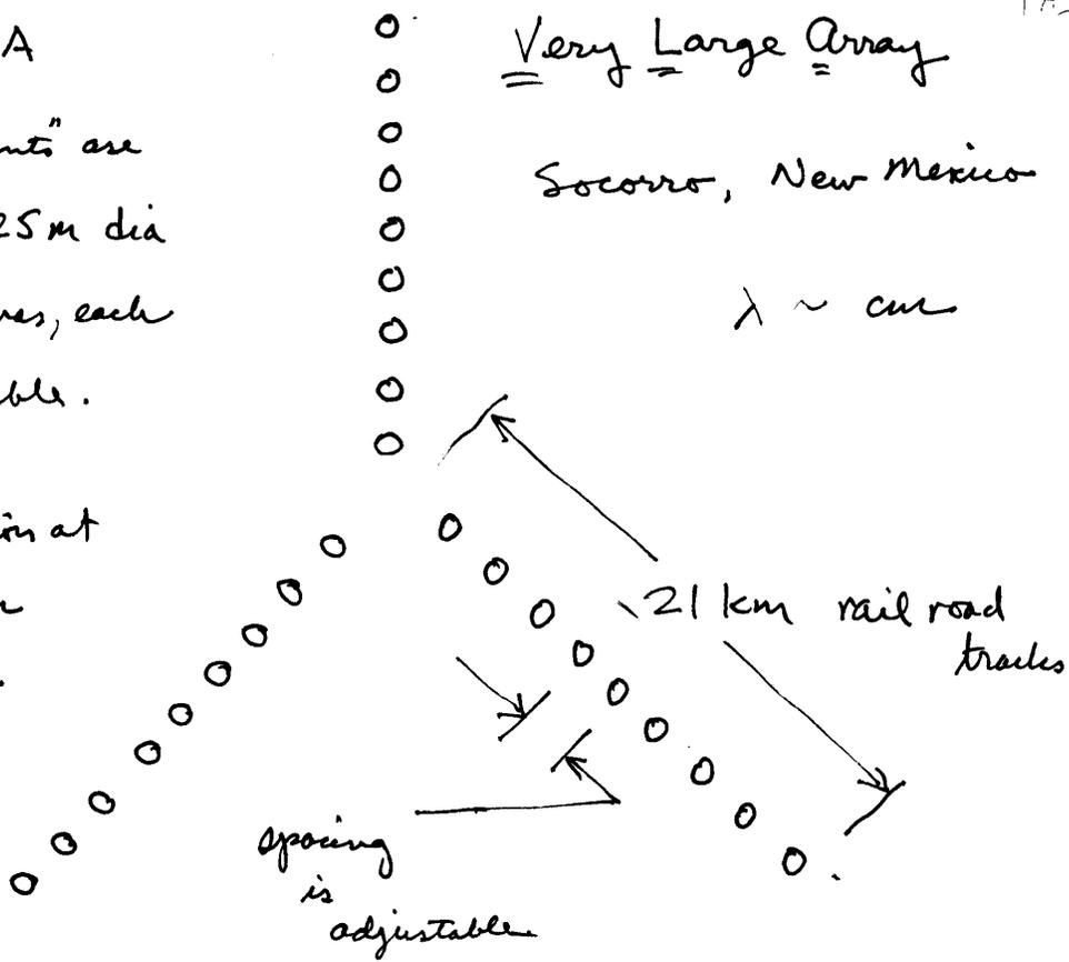
Maximum element spacing is  $2 \times 21 \cdot \sin 60^\circ \approx 36 \text{ km}$
