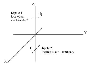
the yz plane, parallel to the y-axis. Dipole 2 lies in the zx plane, parallel to the x-axis. Current  $I_1$  and  $I_2$  are in the sinusoidal steady-state with  $e^{j\omega t}$  time variation.
