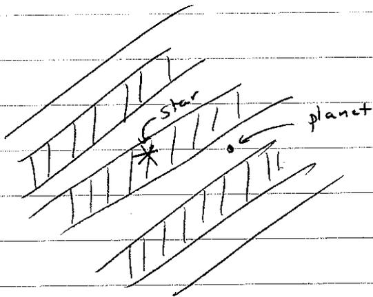
The signal from the star will be a constant intensity, while the signal from the planet will vary as the source is "swept" by the fringe pattern.
