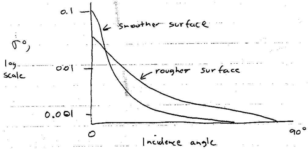
$\sigma^0$  always decreases monotonically with angle. What does this mean for imaging surfaces with terrain?
