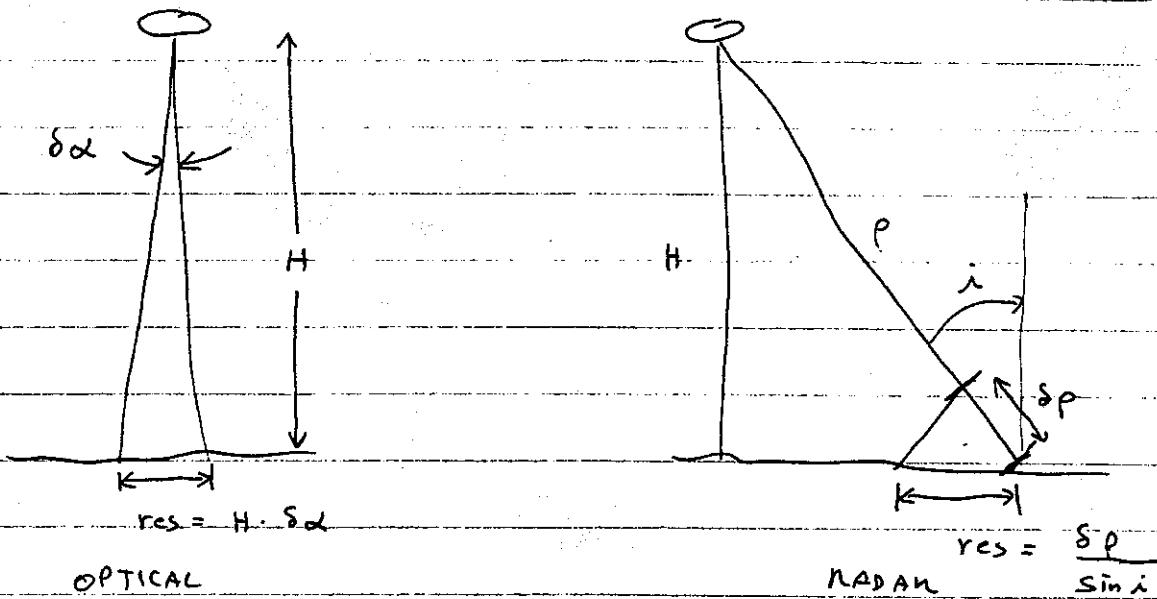
Note that the radar resolution is independent of distance or height, while for the camera-like instrument the resolution is proportional to height. However, for the radar case, as the distance, or range, increases, the signal level drops in strength quickly, make the resulting images low in quality.
