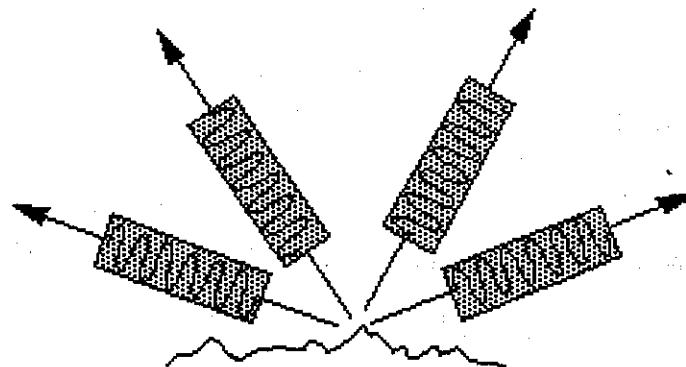
Therefore, one interpretation of brightness in a radar image is roughness, the brighter a surface appears then the rougher it is. And since our scattering is dominated by wavelength-scale structures, we are usually sensitive to objects and roughness from 1cm - 1m in size.
