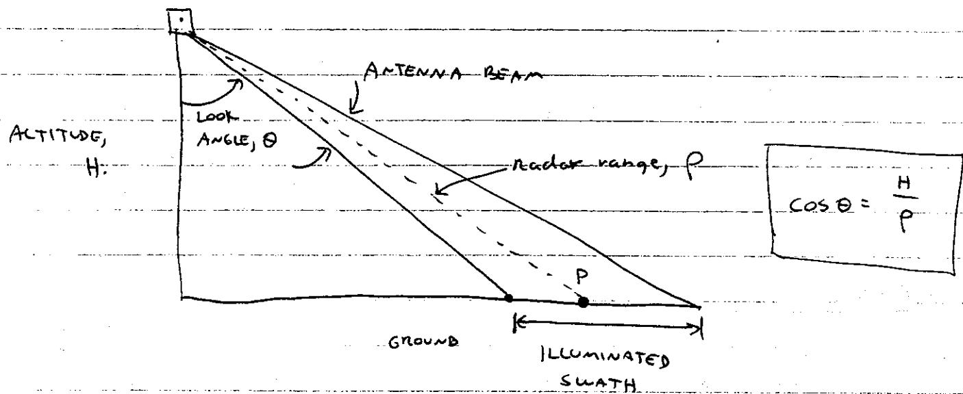
Side-looking geometry, looking into line of flight.
