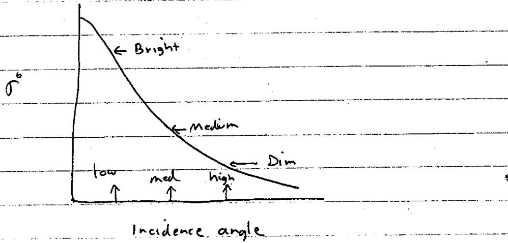
Thus the mountain would appear brighter on the side facing the radar, and dimmer on the side away from the radar, than the surrounding flat terrain. This shading makes radar images quite sensitive to topographic features, so they are quite useful for geologic mapping.
