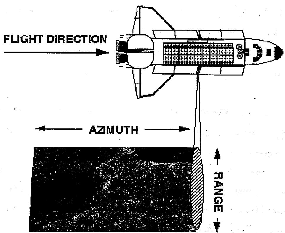
The fundamental measurement a radar system makes is a distance measurement, or range measurement. It is thus quite different than a photograph, which measures the distribution of reflected energy as a function of angle. Even though the final products look similar, they represent very different geometrical perspectives.
