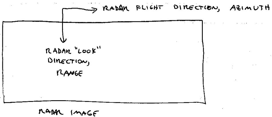
Resolution is given in the range, or across track direction, and the azimuth, or along-track direction.
