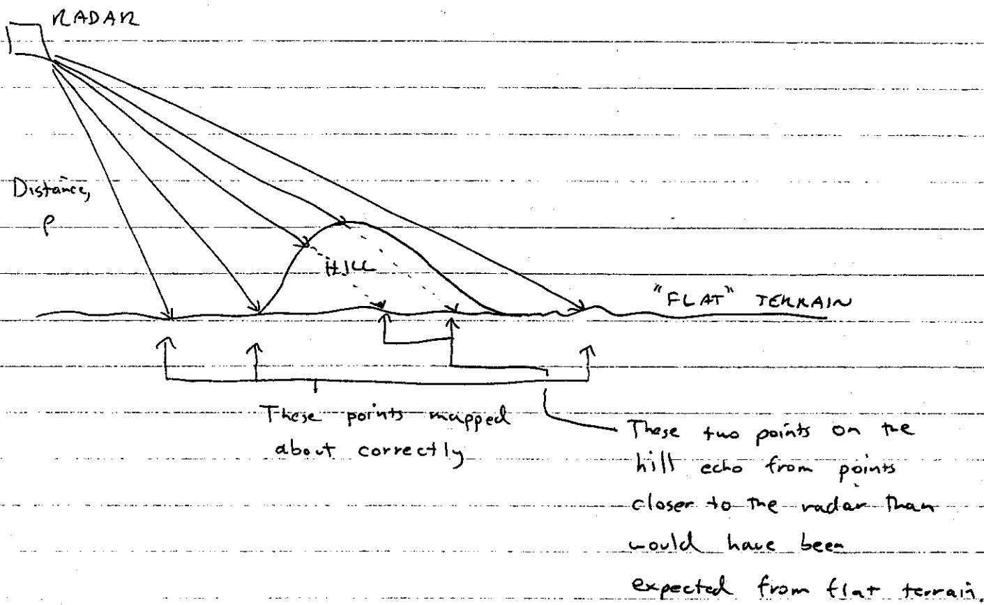
The effect of this is to have the tops of hills appear "closer" to the radar than they would have appeared in the absence of topography. Thus the front sides of hills are foreshortened, while the back sides are stretched out. Combining this geometrical effect with the brightness modulation described earlier gives mountains a distinct and peculiar effect in radar images.
