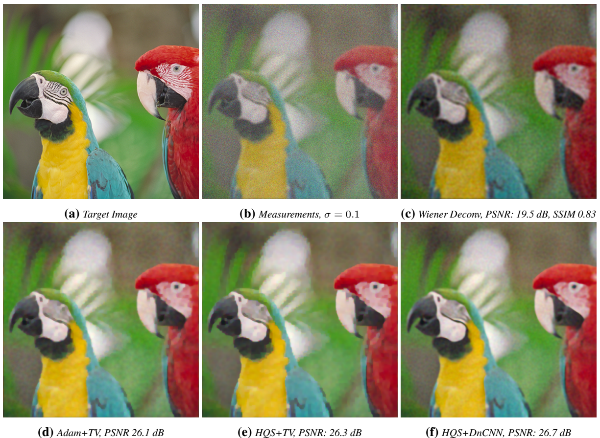
Figure 3: Results. A target image (a) is degraded by blurring it and corrupting the measurements with additive Gaussian noise with \sigma = 0.1 (b). Conventional approaches, including Wiener deconvolution fail at estimating a high-quality reconstruction (c). The Adam solver of the PyTorch package combined with an isotropic TV regularizer does a much better job at recovering the image (d). The HQS solver with a TV regularizer achieves somewhat comparable results to Adam (e). However, HQS is flexible in allowing arbitrary denoisers to be used as regularizers, such as DnCNN. For this example, HQS with DnCNN (f) achieves the best results both qualitative and quantitatively, as measured by the peak signal-to-noise ratio (PSNR).
