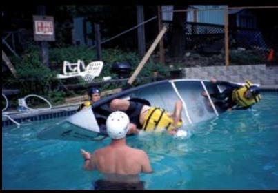
Test subjects are coached during the water portion of the evaluation in which the subject finally gets dumped on the count of three to verify safe egress from the canoe. At least one water safety expert is always on hand for this part of the evaluation.
