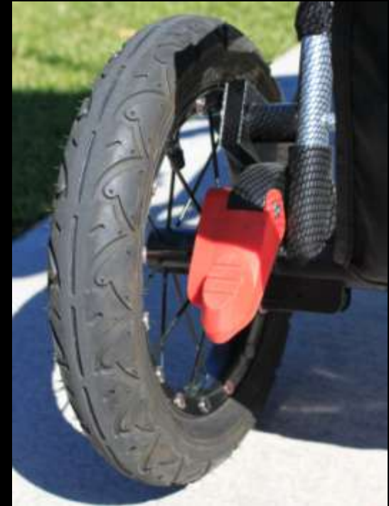
Rear Wheel Distance Encoder with resolution of 0.1 feet
