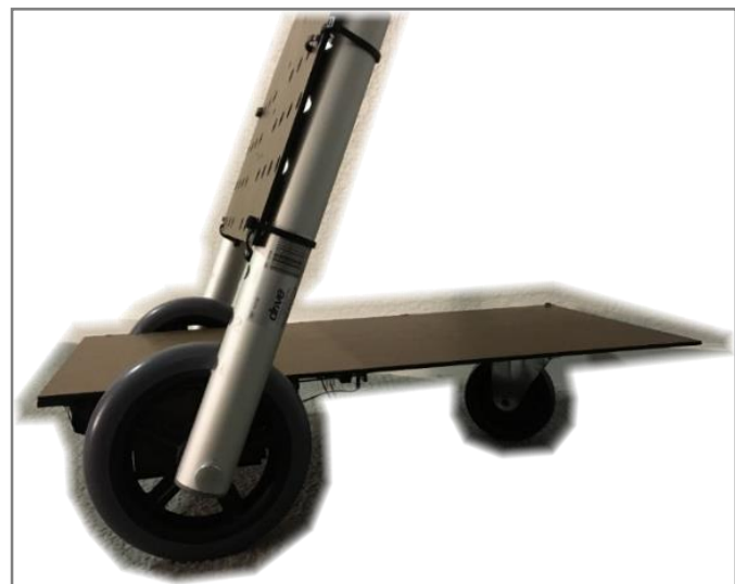
Figure 13. Functional Duro prototype. This prototype allowed for testing and refinement of the various mechanical and electrical components.
