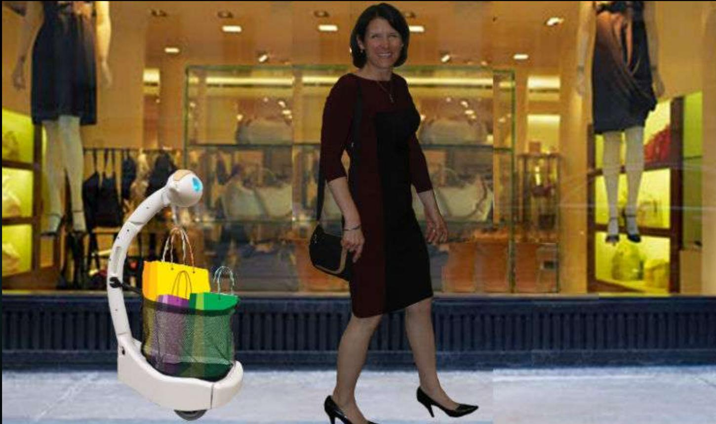
Budgee, the robot assistant, can carry 50 pounds and run up to 10 hours on a charge, and it has sensors on the front and side to avoid obstacles.
