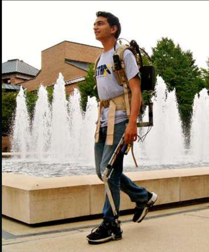
Student team STARX (STrength Augmenting Robotic eXoskeletons) completed its second year, focused on making practical powered exoskeletons that increase the effective strength of the user. This year, they built a new load-bearing exoskeleton called the Lexo. In its finished state, this device will transfer a load of up to 100 lbs off of the user and into the ground so they do not feel the weight. [Link](#)
