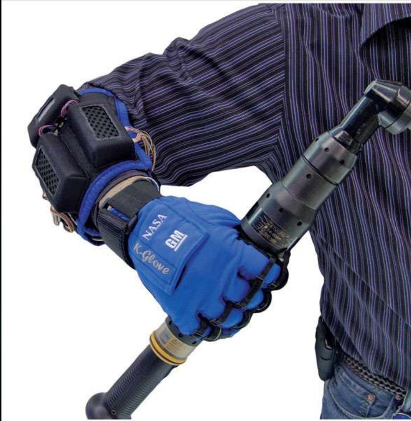
RoboGlove is essentially a wearable exoskeleton gripping tool. It addresses repetitive stress syndrome by reducing the amount of stress involved in an action or process.
