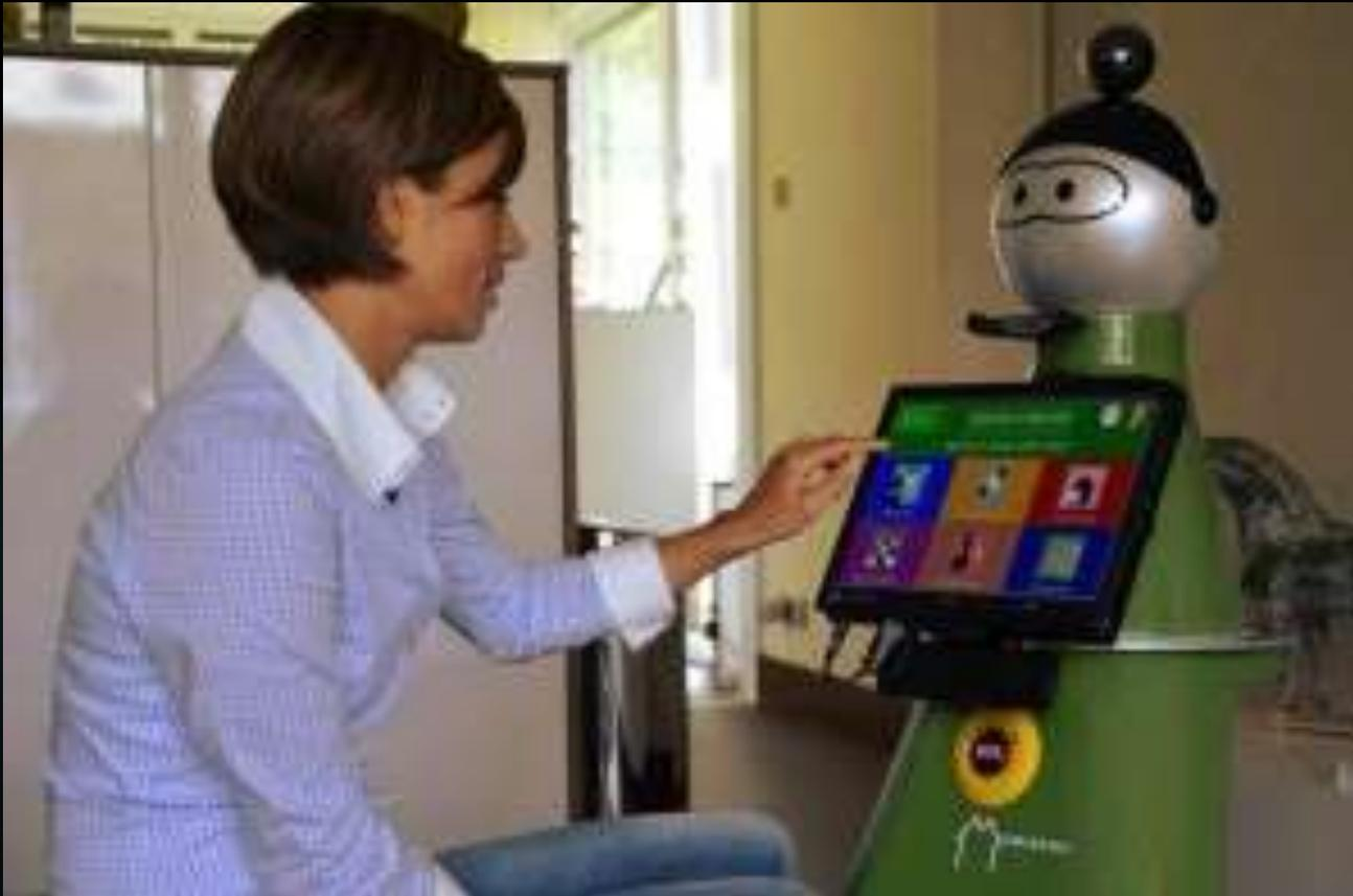
Mobiserv developed a social companion robot – an autonomous robot, containing processing power, data storage capability, various sensors, machine learning / experience gathering / adaptation, a touch screen, speech synthesis, and speech recognition. [Link](#)
