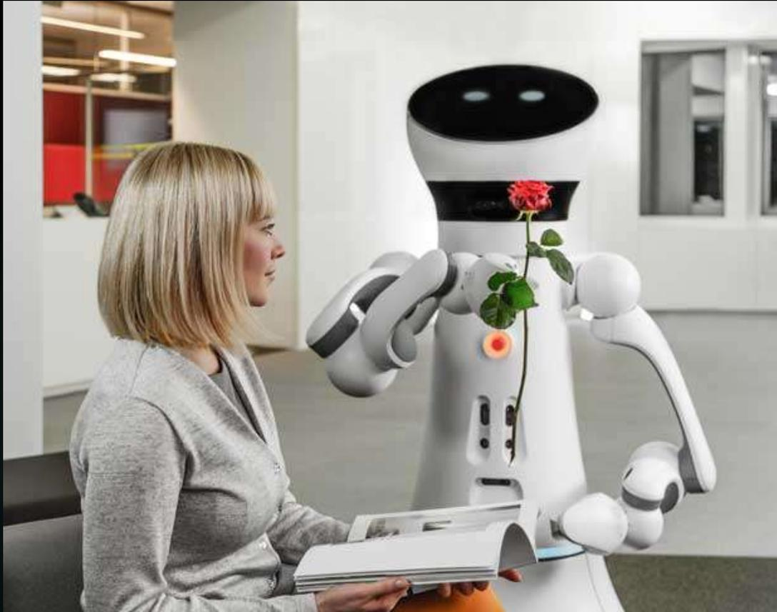
After two decades of refinement, the Care-O-bot 4 robot is constructed out of five modules: base, torso, arms, sensor ring, and head. Each one of these modules can be swapped out depending on what you want the robot to do (and what your budget is).
