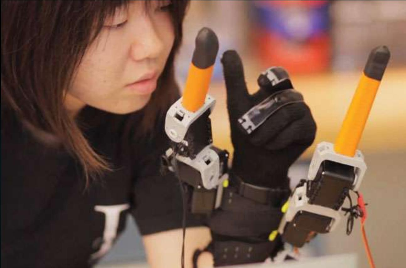
This MIT project added two large fingers to a glove. It lets users do things like hold an object with a couple of fingers while using the others to perform another job such as adding salt to a cup of liquid or opening the top of a jar.
