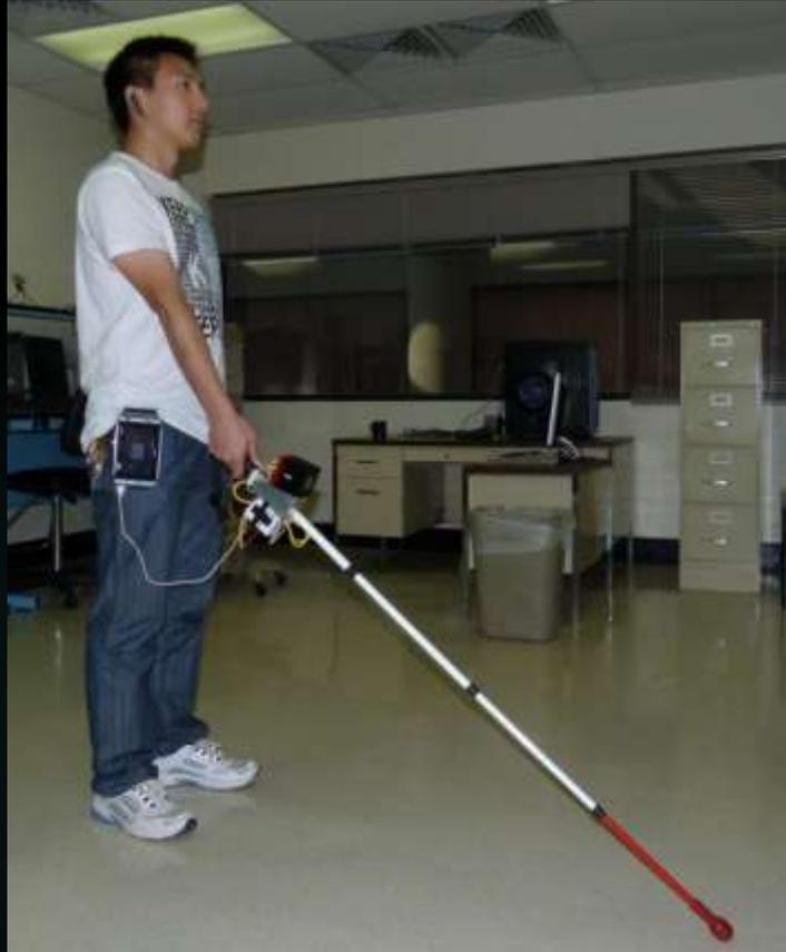
A co-robotic cane developed at the University of Arkansas at Little Rock promises to make life easier for blind people to navigate. The cameras detect obstacles in the user's path and provide audio feedback to facilitate safe travel. In addition, the cane provides guidance via a rolling tip that points in the proper direction.
