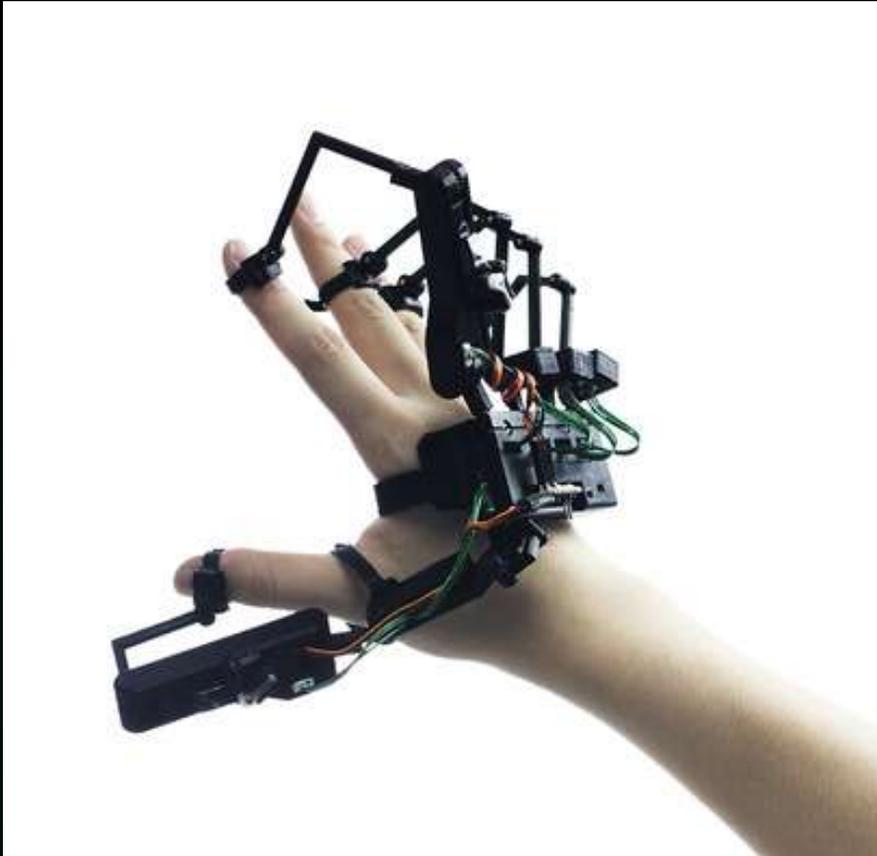
China's Dexta Robotics has created an exoskeleton for hands to allow gamers to touch the digital world. The Dexmo is a mechanical exoskeleton system that features force feedback, rotational sensors, and injection molded parts. Applications include medical rehabilitation. [Link](#)
