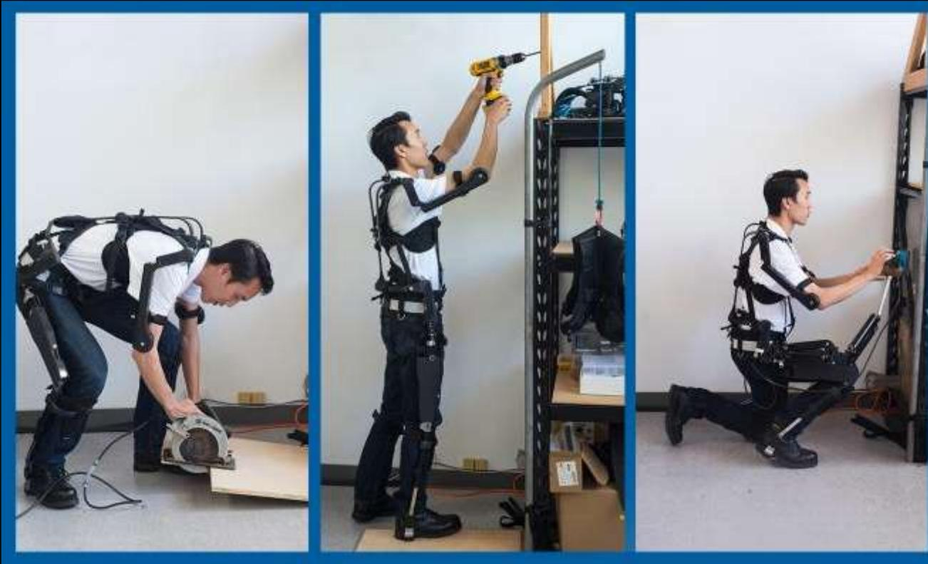
MAX (Modular Agile eXoskeleton) is a workplace exoskeleton in three modules that allows workers to complete shoulder, lower back and leg-intensive tasks with reduced injury risk. [Link](#)
