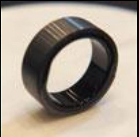
For people with limited mobility, **Lotus** is a patented wearable ring to control objects at home by pointing. With Lotus, control anything a wall switch controls, like lights and fans - and even the TV - from wherever you are in the room. No rewiring, no apps, no internet.
