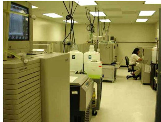
AB slab gel sequencers (370, 373, 377) Fluorescent sequencing 1990-1999 6 runs/day 96 reads/run 500 bp/read 288,000 bp/day
