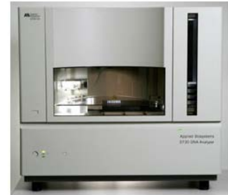
AB capillary sequencers (3700, 3730) 1998-now 24 runs/day 96 reads/run 550 – 1,000 bp/read 1-2 million bp/day
