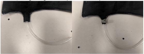
11. Try inflating the bladder and note any leaks. Use the iron to reseal any sections that are leaking.
