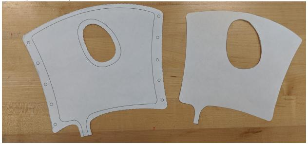
2. Use the larger template to trace out the pattern on the non-shiny (matte) side of the ripstop nylon (use the silver paint pens for best results). **Flip the template over and trace a second pattern.** You need two mirrored pieces (see picture below) so that they will align when the heat-weldable sides are touching.
