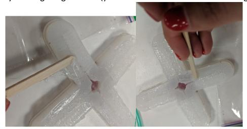
9. Press the gripper silicone onto the silicone sheet. Make sure all of the edges are pressed down. You can use a weight or the mold to help the pieces together while they glue. You should see some Silpoxy get squeezed out.
