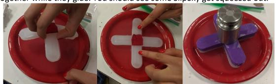
10. Make sure the pieces are firmly pressed together (Silpoxy might squeeze out the edges of the gripper, this is ok) and let sit for at least 30 minutes.
