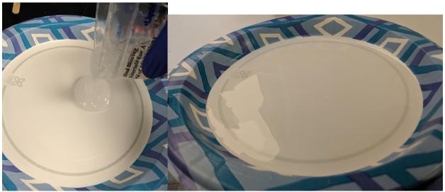
6. Place the two plates on level surfaces to cure for at least 4 hours. **(END HERE ON FIRST DAY)**
