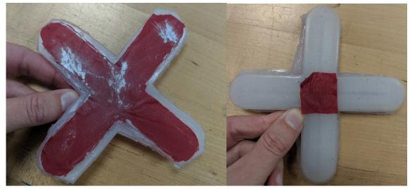
15. Poke a small hole in the side of the gripper between two of the "fingers" (use the tweezers or a needle)
