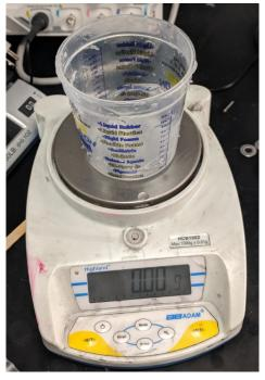
2. Measure out equal parts of EcoFlex 00-30 Part A and EcoFlex 00-30 Part B by weight, **using about 100 g total (i.e. 50 g of each part)**. First, measure out one part to approximately half the desired weight and then measure the second part to match.
