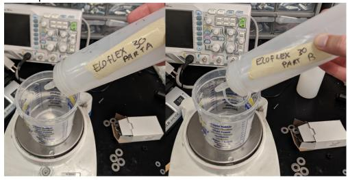
3. Mix the two parts together well using the mixing stick.
