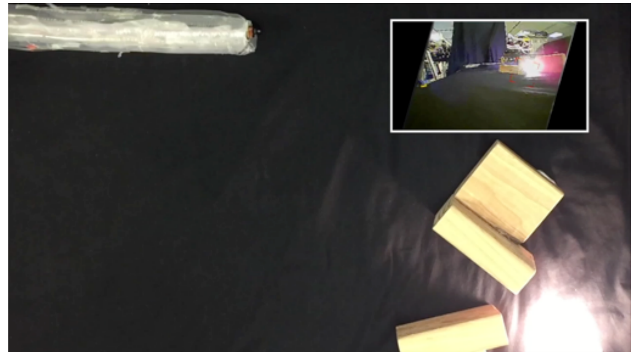
active steering using tip-mounted camera
