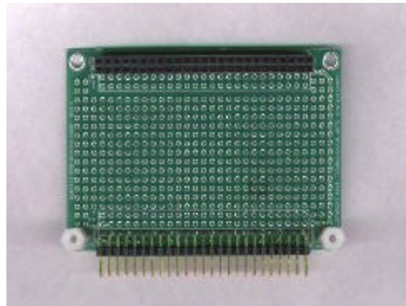
Figure 31. Technological Arts Adapt12 prototyping card (Adapt12PRO1). [22]
