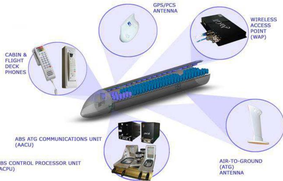
Figure 19 - Elements of Wi-Fi technology which interacts with the aircraft's architecture [25]
