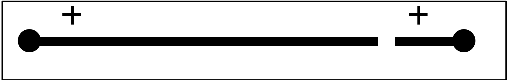
Mask for 7 \mu\text{m} -thick Positive Resist Layer
