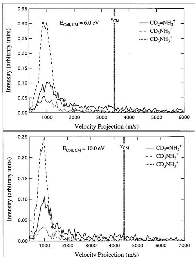
FIG. 11. Laboratory-frame velocity histograms for  $\text{CD}_2=\text{NH}_2^+$ ,  $\text{CD}_3\text{NH}_2^+$ , and  $\text{CD}_3\text{NH}_3^+$  for center-of-mass collision energies of 6.0 and 10 eV. The velocity of the center-of-mass is also shown.
