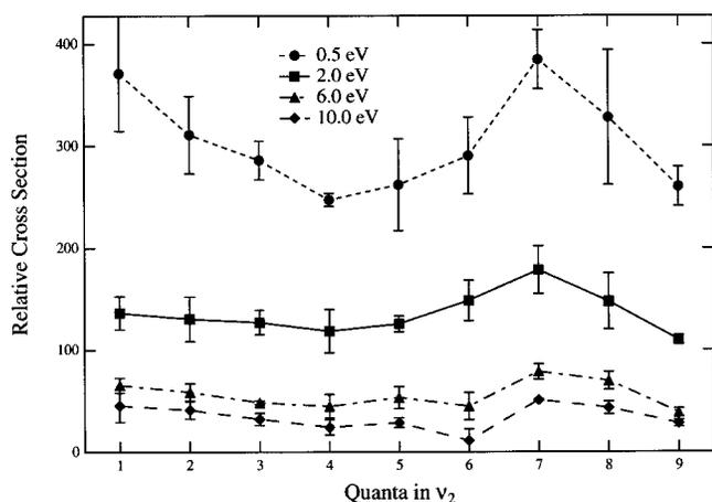
FIG. 9. Relative reaction cross sections (arbitrary units) for the formation of  $\text{CD}_3\text{NH}_3^+$  as a function of ammonia-ion vibrational state (quanta in  $\nu_2$ ) at the center-of-mass collision energies of 0.5, 2, 6, and 10 eV. The error bars represent one standard deviation ( $\pm s$ ).
