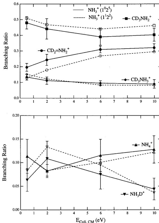
FIG. 12. Product branching ratios as a function of center-of-mass collision energy. Reactions of both  $\text{NH}_3^+$  ( $1^02^5$ ) ( $E_{\text{int}}=0.60$  eV) and  $\text{NH}_3^+$  ( $1^12^2$ ) ( $E_{\text{int}}=0.63$  eV) are shown. Error bars represent the pooled standard deviation for both sets of data multiplied by Student's  $t$  at a 95% confidence level ( $t_{s_{\text{pooled}}}$ ).
