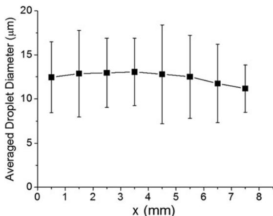
**Fig. 5.** Average diameter of pure-water droplets in the microdroplet fusion mass spectrometry as a function of the distance ( $x$ ). Few noticeable differences were observed in the average size of microdroplets up to the distance of about 7 mm from the droplet fusion center. All kinetic measurements shown in Fig. 4 are performed at distances of 4 mm or less.
