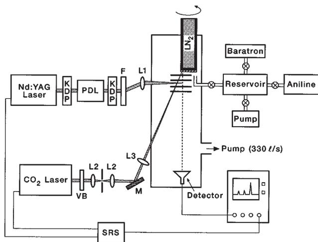
FIG. 1. Schematic of the apparatus used to study the ir laser-induced thermal desorption mechanism. Some abbreviations are F=filter, L=lenses, LN<sub>2</sub>=liquid nitrogen, M=gold mirror, PDL=pulsed dye laser, SRS=pulse generator, VB=Venetian blind.
