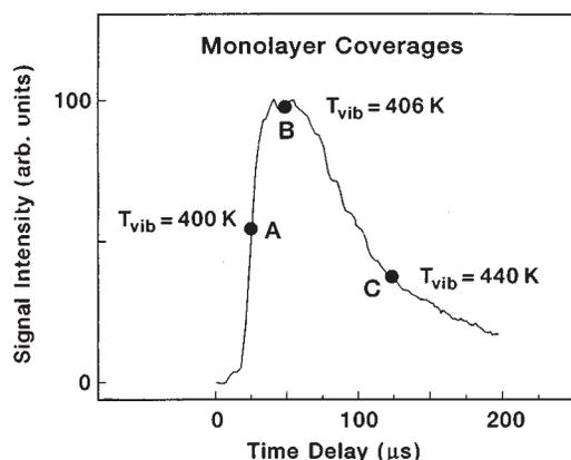
FIG. 3. Vibrational temperatures of desorbed aniline-*d7*. Vibrational temperatures are recorded at three points along a profile from monolayer coverage: A, B, and C. Similar temperature values are observed for the three points, demonstrating that collisions between desorbing molecules do not affect (i.e., cool) the vibrational energy distributions.
