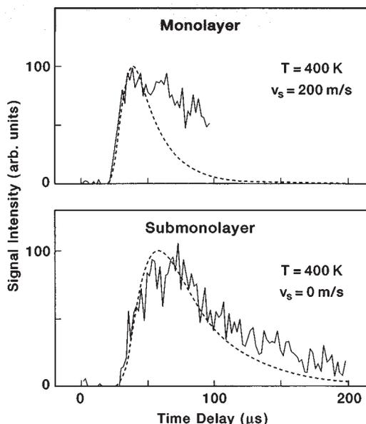
FIG. 2. TOF profiles of desorbed aniline-*d*7. Submonolayer coverages correspond to a Maxwell–Boltzmann distribution with a temperature of 400 K. Monolayer coverages correspond to a Maxwell–Boltzmann distribution with a stream velocity of 200 m/s and a temperature of 400 K. The stream velocity accounts for collisions between desorbing molecules that increase the net speed of the distribution in the direction of the surface normal.
