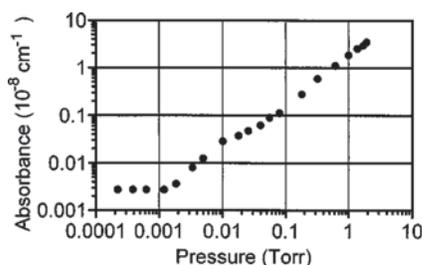
FIG. 5. Observed absorbance loss plotted as a function of CO<sub>2</sub> pressure with the laser frequency set at the peak of the CO<sub>2</sub> absorption feature.
