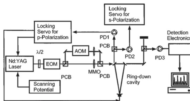
FIG. 1. Schematic diagram of laser-locked CRDS system. Abbreviations are as follows: EOM is the electro-optic modulator,  $\lambda/2$  is the half-wave plate, PCB is the polarizing cube beamsplitter, AOM is the acousto-optic modulator, PD1, PD2, and PD3 are the photodetectors used to detect reflected  $p$ - and  $s$ -polarized beams and transmitted  $s$ -polarized light, respectively.
