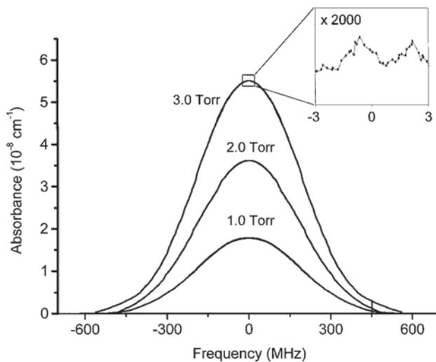
FIG. 4. Absorption spectra of CO<sub>2</sub> obtained at 3.0, 2.0, and 1.0 Torr using the CRDS system and analog detection system described here. Noise on the scan obtained at 3.0 Torr is shown on an expanded scale.
