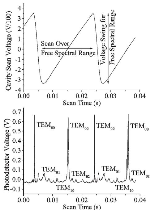
Fig. 2. Optical resonator transmission (bottom) as a function of frequency when the cavity length is swept in time, with a voltage sweep (top).
