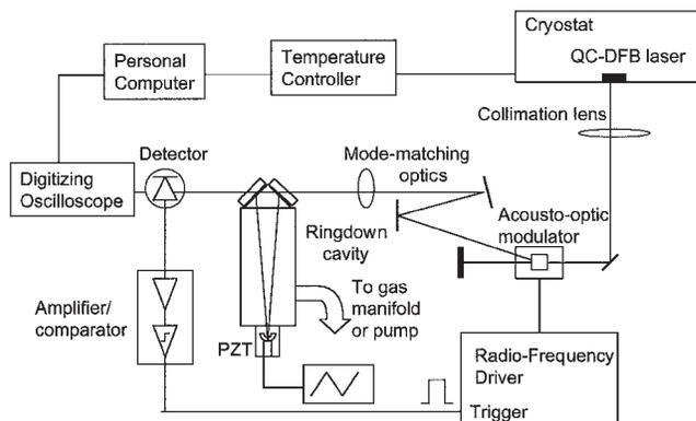
Fig. 1. Block diagram of the CDRS.<sup>9</sup> PZT, piezoelectric transducer.
