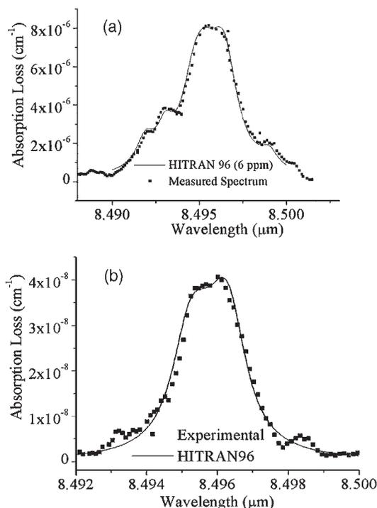
Fig. 4. (a) Single-shot spectrum of 4-ppmv ammonia in nitrogen compared with a spectrum generated by HITRAN96. (b) Averaged spectra of 10-ppbv ammonia at STP.
