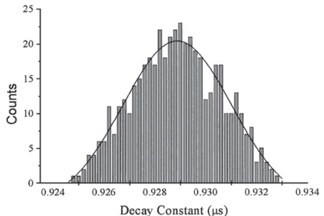
Fig. 3. Single-shot statistics for 500 shots, for a stationary wavelength ( $\lambda = 8.45 \mu\text{m}$  at  $T = 45.3 \text{ K}$ ) and a ringdown cavity filled with nitrogen.
