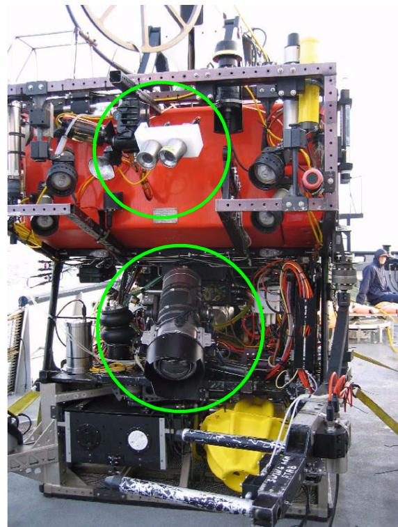
**Figure 1** The ROV *Ventana*, configured with cameras for midwater tracking (circled, top center). The high definition science camera is indicated in the lower circle.
