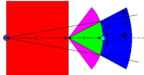
**Figure 5** Parameterization of camera view of target of diameter  $D$  with camera with half-angle field-of-view  $\omega$ . Camera is located  $L$  m from the center of the vehicle. View is from above, looking down at vehicle, and camera as illustrated has no pan or tilt angles. Maximum allowable pointing error is given by equation (4).
