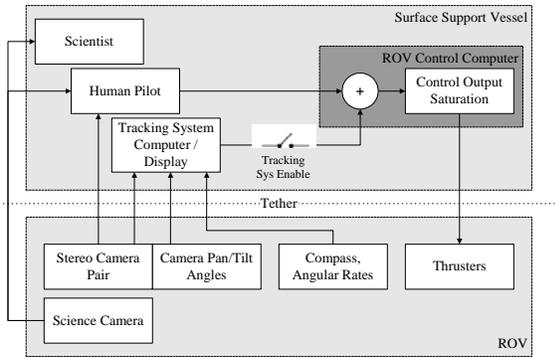
**Figure 2** Block diagram of tracking system hardware and its interactions with the human ROV pilot and scientist.
