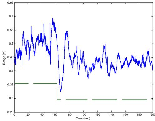
**Figure 10** Range control while tracking an *Aegina* jellyfish. The lower line (dotted) indicates the range reference value. (Offset is due to tether disturbance forces and the lack of an integral control term during this experiment.)
