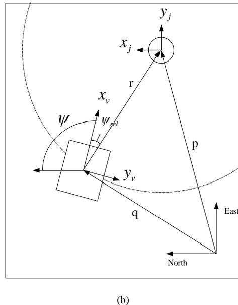
**Figure 3** Vision-based sensing (a) coupled with cylindrical control system (b) for tracking of midwater ocean animals. In (a), subscripts indicate frames as water (w), sensor (s), vehicle (v) and jelly (j). In (b), the vehicle is indicated by the rectangle, the target jelly by the circle.
