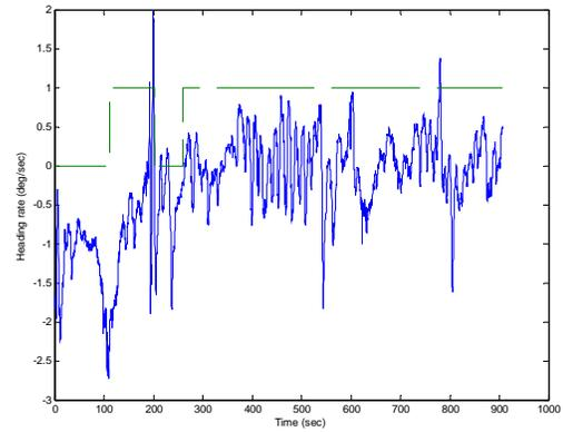
**Figure 11** Demonstration of heading hold performance while tracking a *Solmissus* jellyfish. The solid line is measured yaw rate of the tracking vehicle. The dotted line indicates heading hold on (1) or off (0).
