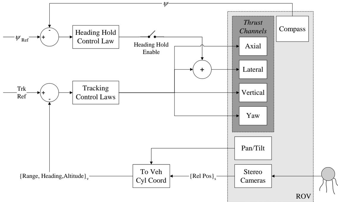
**Figure 9** Control architecture of tracking system, modified to include an optional heading hold loop to stabilize the vehicle's position on the circle about the target.
