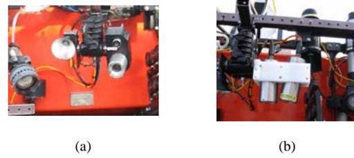
**Figure 7** Camera sets for relative position sensing: (a) vertically aligned parallel wide angle and narrow angle cameras, (b) horizontally aligned and converging narrow angle cameras.
