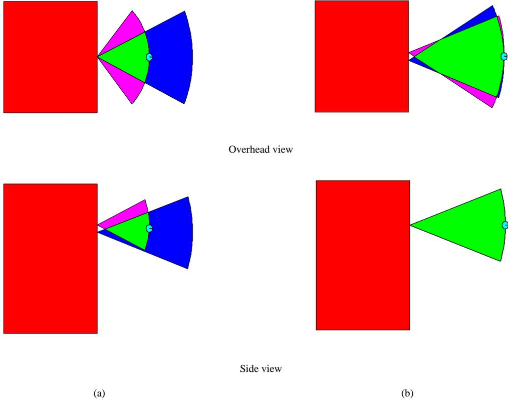
**Figure 6** Stereo vision cone overlap for (a) a wide/narrow camera pair aligned vertically and parallel and (b) a narrow/narrow camera pair horizontally aligned and converging at a 10 degree angle. Both illustrate the maximum range to target based on the worst case  $O_{\min}$  constraint for the camera set. The stereo vision sensor was redesigned from the configuration of (a) to that of (b) to increase the volume in which the target can be seen.
