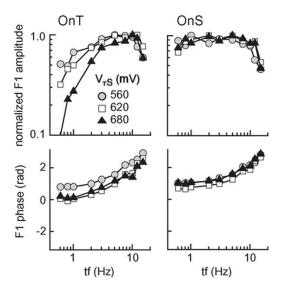
Fig. 10. Changing the open loop gain. Temporal frequency responses of chip OnT and OnS GCs to a 0.2192 cyc/deg drifting sinusoidal grating. Profiles are shown for three different values of  $V_{\tau s}$ , which determines the open loop gain, g. Increasing  $V_{\tau s}$  above the dc unity value of 620 mV increases the open-loop gain, g, increasing the system's corner frequency. Phase data are shown on the bottom for the three different  $V_{\tau s}$  conditions.
