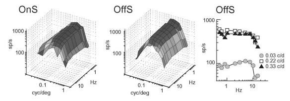
Fig. 7. Sustained cell spatiotemporal response. Three dimensional plots of chip sustained GC responses, which reflect activity at the bipolar terminal, to horizontally drifting sinusoids of different spatial and temporal frequencies. OFF sustained GC temporal frequency responses are shown on the right, in two dimensions, for three different spatial frequencies. Chip sustained cells are bandpass in space for all temporal frequencies.
