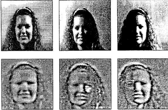
**Figure 7. CCD Camera (top row) versus OPL imager chip (bottom row) under variable lighting. The CCD camera performs global AGC whereas the OPL chip performs local AGC and bandpass-filtering.**
