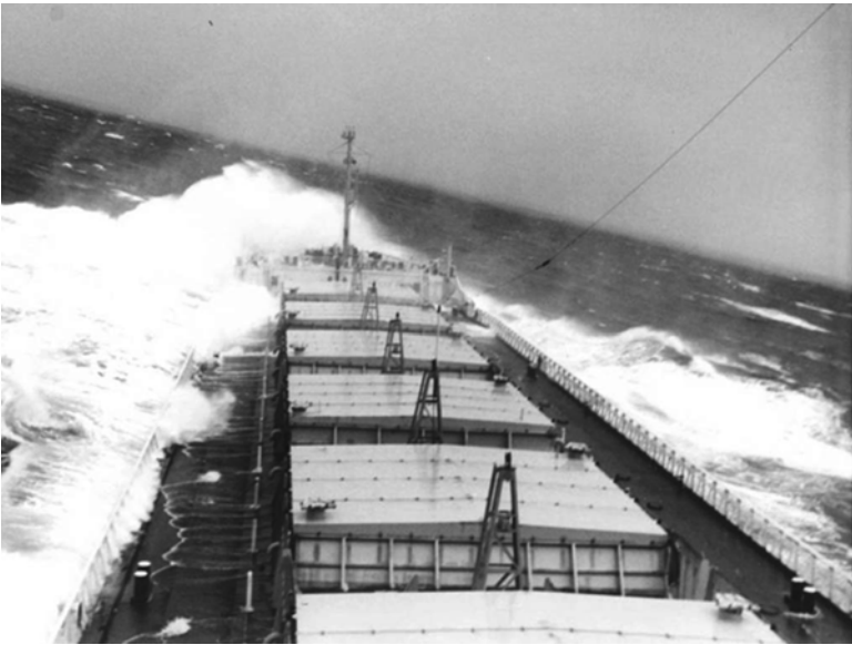
Fig. 13 Vessel in heavy weather conditions, waves in transversal effect (Source: Cornelius de Keyzer, Master Mariner, Port of Rotterdam, the Netherlands)
