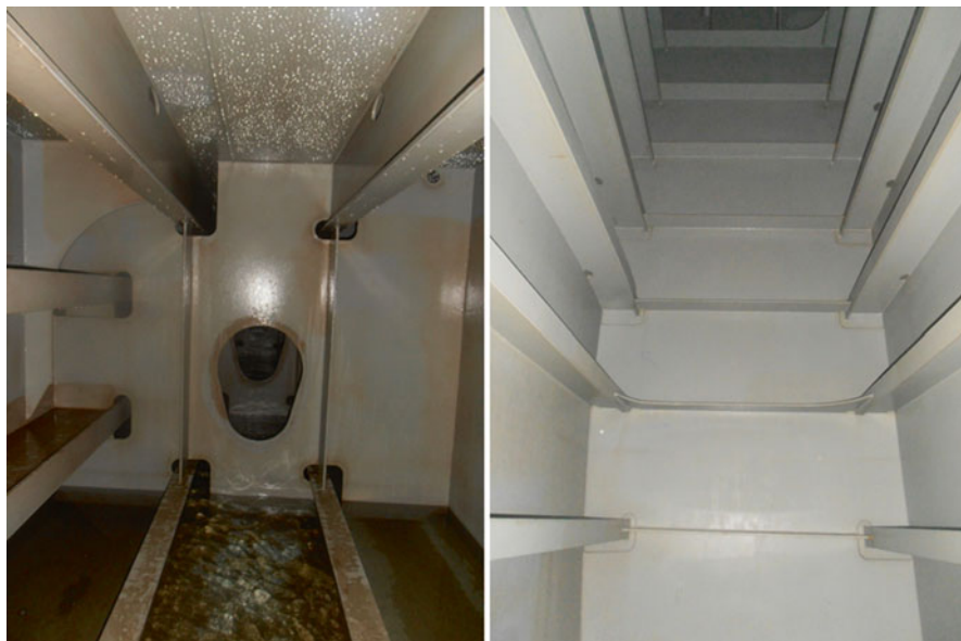
Fig. 2 Interior of a DBT ( left ) and ST ( right ) ballast tank on a bulk carrier (Photos: Guy Mali)
