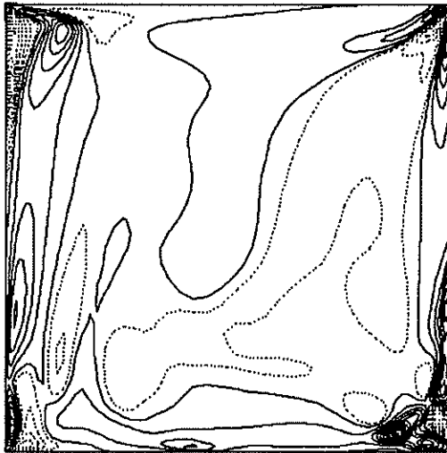
FIGURE 4B. Contours of computed C near one of the side walls. Dotted lines represent negative values.
