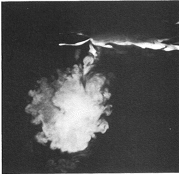
FIGURE 3. Jet sheet ejected from the wide gap at U_e \approx 1 m/s, when the vortex generator is pointed in the downstream direction.
