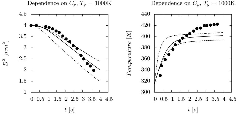
FIGURE 2. Case 3. Sensitivity of decane drop diameter (left) and drop temperature (right) to gas composition used to evaluate  $C_p$ . Experiments from Wong & Lin (1992) ( $\bullet \bullet \bullet$ ) are compared with model solutions in which  $C_p$  is evaluated as  $C_p = Y_{ref}C_{p,f} + (1 - Y_{ref})C_{p,g}$  using a gas composition of  $Y_{ref} = (2/3)Y_{d,s} + (1/3)\tilde{Y}_f$  (—),  $Y_{ref} = 0$  (---), or  $Y_{ref} = 1$  (- · -).
