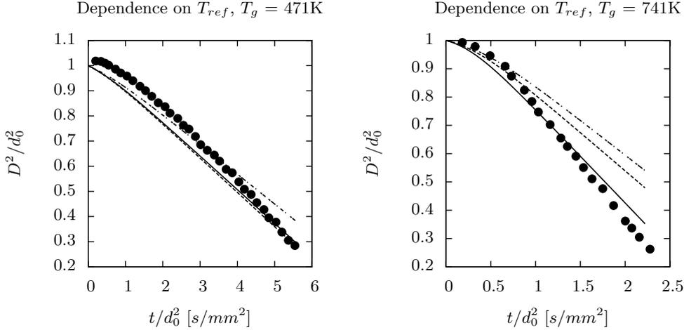
FIGURE 3. Cases 4 (left) and 5 (right). Sensitivity of heptane drop diameter ( $D$ ) to the temperature used to evaluate  $C_p$ . Experiments from Nomura *et al.* (1996) ( $\bullet \bullet \bullet$ ) are compared with model solutions in which  $C_p$  is calculated at a temperature of  $T_{ref} = (2/3)T_d + (1/3)\tilde{T}_g$  (—);  $T_{ref} = T_{b,atm}$  (---);  $T_{ref} = T_d$  ( $\cdot - \cdot$ ).
