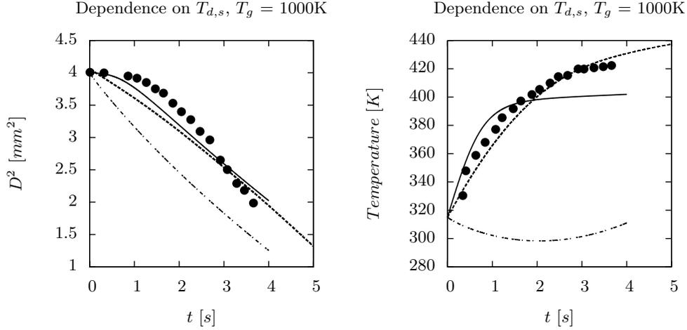
FIGURE 6. Case 9. Sensitivity of decane drop diameter to the temperature  $T_{d,s}$ . Experiments from Wong & Lin (1992) ( $\bullet \bullet \bullet$ ) are compared with model solutions in which  $T_{d,s}$  is calculated by assuming  $T_{d,s} = T_d$  (—), by calculating  $T_{d,s}$  from Eq. (2.14) so that  $B_M = B_T$  ( $\cdot - \cdot$ ), or by calculating  $T_{d,s}$  from Eq. (2.13) so that  $(1 + B_M)^\phi = (1 + B_T)$  (---).
