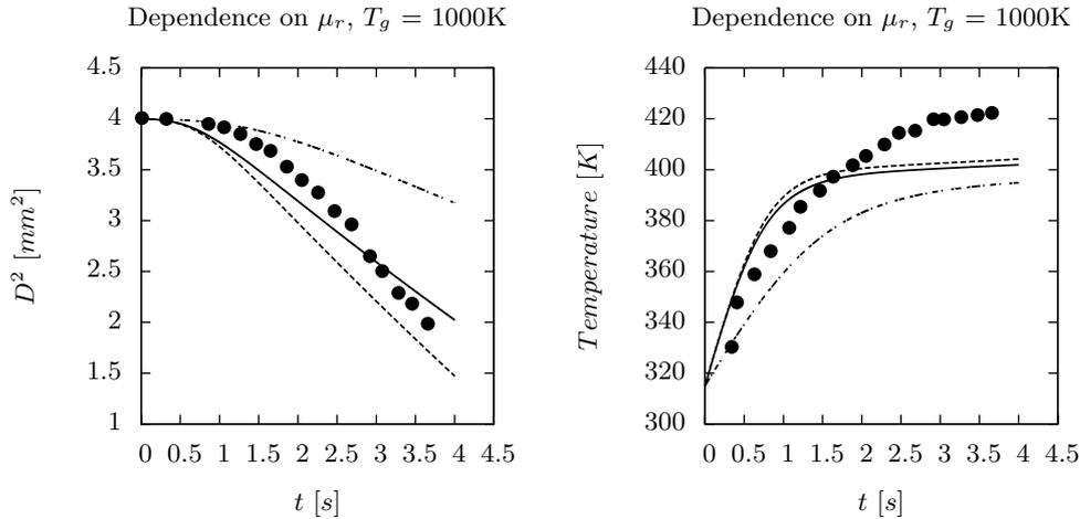
FIGURE 5. Case 8. Sensitivity of decane drop diameter (left) and drop temperature (right) to the temperature used to evaluate  $\mu_r$ . Experiments from Wong & Lin (1992) ( $\bullet \bullet \bullet$ ) are compared with model solutions in which  $\mu_r$  is calculated at a reference mole fraction of  $X_{ref} = (2/3)X_{d,s} + (1/3)\tilde{X}_f$  (—);  $X_{ref} = 0$  (---);  $X_{ref} = 1$  (-.-).
