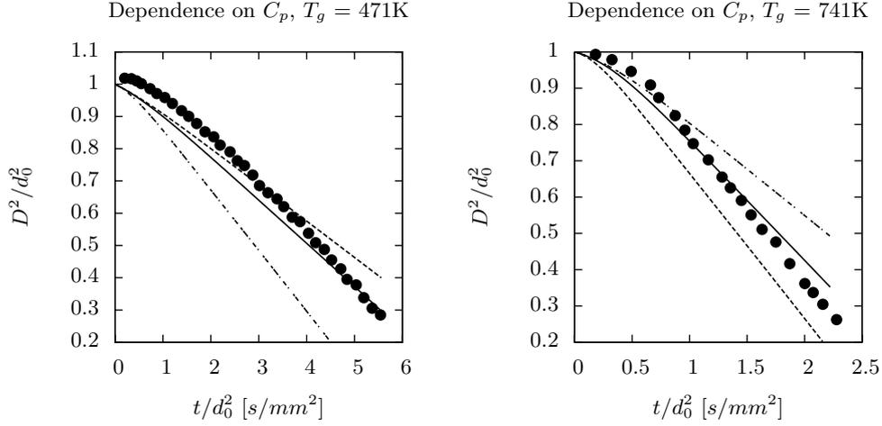
FIGURE 1. Cases 1 (left) and 2 (right). Sensitivity of heptane drop diameter ( $D$ ) to the gas composition used to evaluate  $C_p$ . Experiments from Nomura *et al.* (1996) ( $\bullet \bullet \bullet$ ) are compared with model solutions in which  $C_p$  is evaluated as  $C_p = Y_{ref}C_{p,f} + (1 - Y_{ref})C_{p,g}$  using a gas composition of  $Y_{ref} = (2/3)Y_{d,s} + (1/3)\tilde{Y}_f$  (—),  $Y_{ref} = 0$  (---), or  $Y_{ref} = 1$  (- · -).
