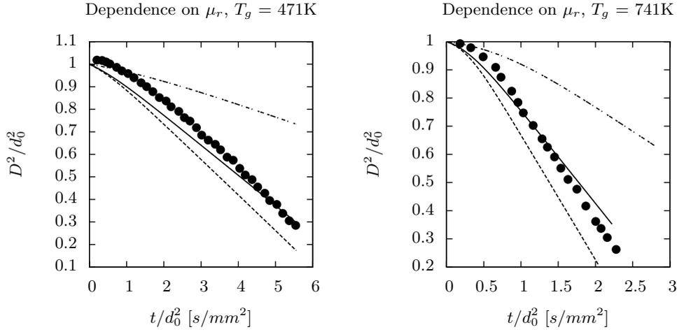
FIGURE 4. Cases 6 (left) and 7 (right). Sensitivity of heptane drop diameter to the temperature used to evaluate  $\mu_r$ . Experiments from Nomura *et al.* (1996) ( $\bullet \bullet \bullet$ ) are compared with model solutions in which  $\mu_r$  is calculated at a reference mole fraction of  $X_{ref} = (2/3)X_{d,s} + (1/3)\tilde{X}_f$  (—);  $X_{ref} = 0$  (---);  $X_{ref} = 1$  (-.-).
