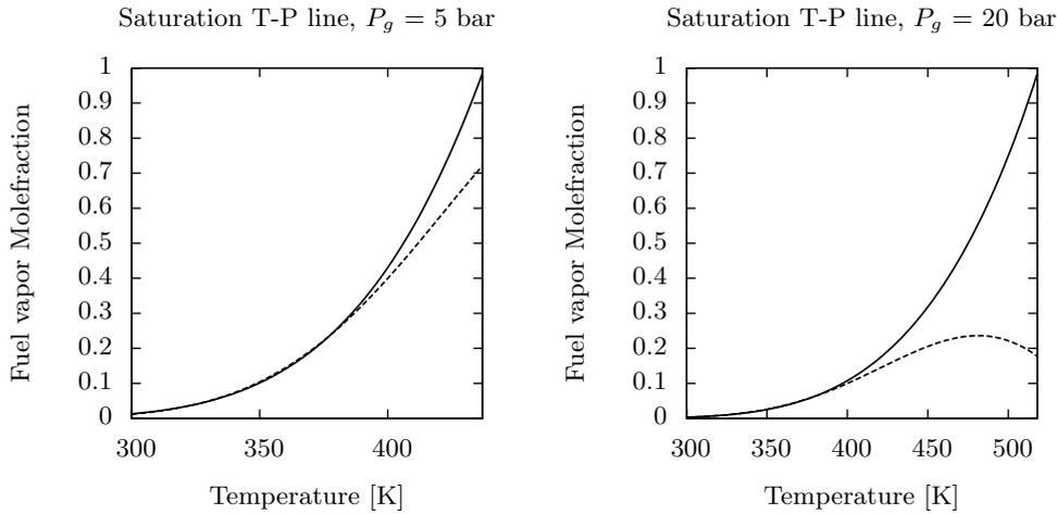
FIGURE 7. Performance of the Clausius-Clapeyron approximation. The saturation fuel mole fraction that is calculated from the saturation pressure in the NIST web book (—) is compared with the saturation fuel mole fraction calculated from the Clausius-Clapeyron expression in Eq. (2.11) (---).
