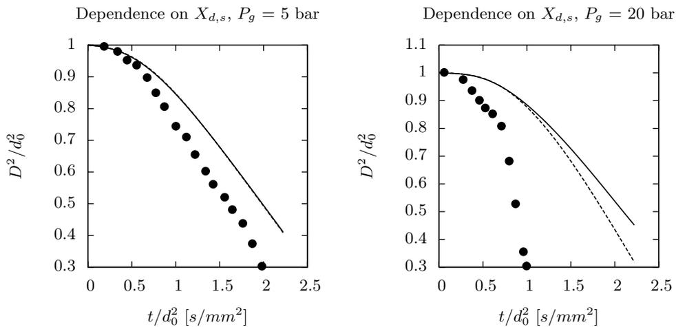
FIGURE 8. Cases 10 (left) and 11 (right). Sensitivity of heptane drop diameter to the saturation mole fraction  $X_{d,s}$  used in evaluating  $B_M$ . Experiments from Nomura *et al.* (1996) (●●●) are compared with model solutions where  $X_{d,s}$  is taken from Clausius-Clapeyron in Eq. (2.11) (—) or directly from the NIST web book saturation pressure (---).
