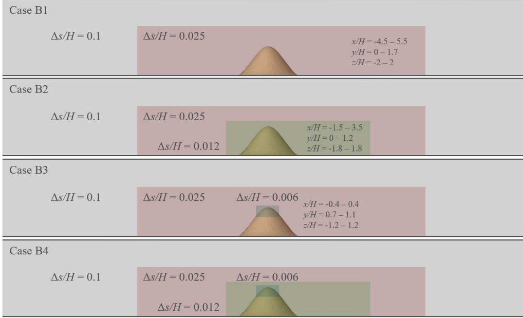
FIGURE 6. Schematic diagram of the mesh refinement.
