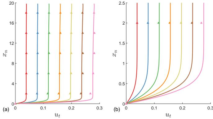
FIGURE 4. Comparison of boundary layer profiles between coarse FSWM (symbols) and DNS calculations (solid lines). From left to right, the stations correspond to  $x_t = 17.50, 35.50, 53.50, 71.50, 89.50, 107.50$  and  $125.50$ . (a) Entire domain. (b) Zoomed-in perspective.
