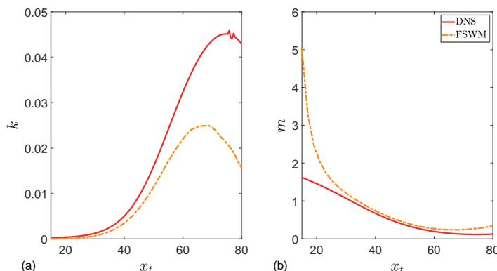
FIGURE 10. A comparison of the DNS (solid line) and the FSWM simulation (dashed line) of the Falkner-Skan variables (a)  $k$  and (b)  $m$ .
