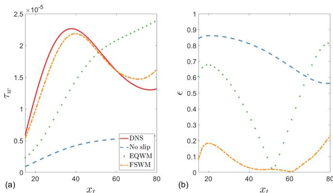
FIGURE 9. (a) Wall stress predicted by different boundary conditions for the coarse simulation: no slip (dashed line), EQWM (dotted line), and FSWM (dot-dashed line). The DNS (solid line) is given for reference. (b) The associated error.
