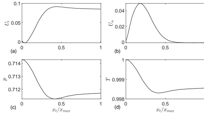
FIGURE 7. Inlet profiles used to initialize the spatially varying pressure-gradient boundary layer flow case in charLES. (a) wall-tangential velocity, (b) wall-normal velocity, (c) pressure, and (d) temperature.
