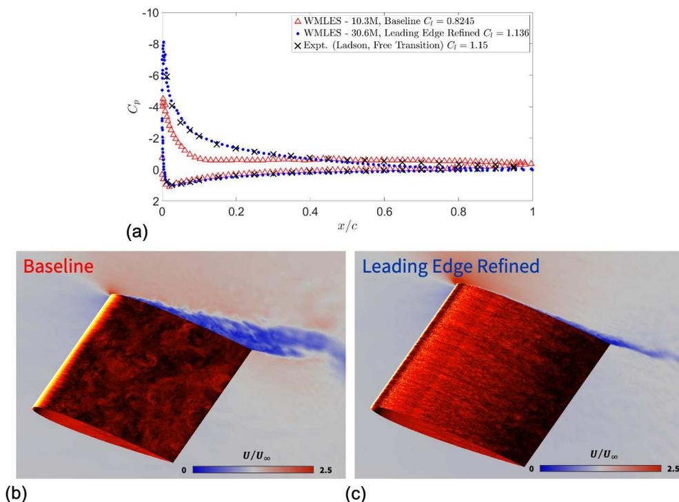
FIGURE 1. Effect of leading-edge resolution on WMLES of the NACA0012 at  $AoA = 15$  degrees,  $Re_c = 3M$ , and  $Ma_\infty = 0.3$ , adapted from Goc *et al.* (2020). (a) Sectional surface pressure coefficient for the two grids compared with experimental data from Ladson *et al.* (1987). (b) WMLES baseline grid resolution (10M control volumes). (c) WMLES with  $\times 4$  leading-edge grid resolution refinement (30.6M).
