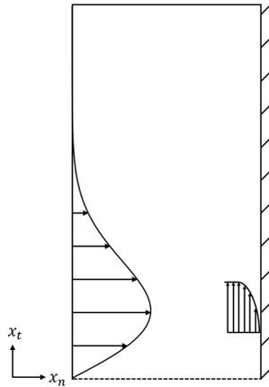
FIGURE 6. Schematic of a spatially varying pressure-gradient boundary layer flow.
