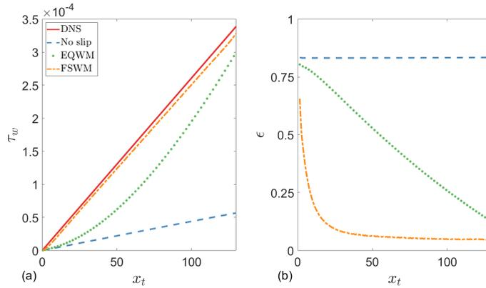
FIGURE 5. (a) Wall stress predicted by different boundary conditions for the coarse simulation: no slip (dashed line), EQWM (dotted line), and FSWM (dot-dashed line). The DNS (solid line) is given for reference. (b) The associated error.
