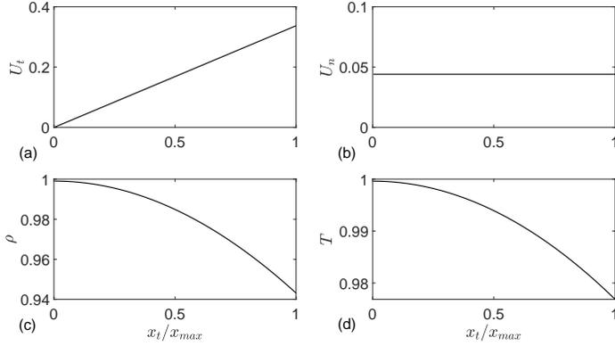
FIGURE 3. Inlet profiles used to initialize the stagnation flow case in charLES. The profiles are (a) wall-tangential velocity, (b) wall-normal velocity, (c) density, and (d) temperature.
