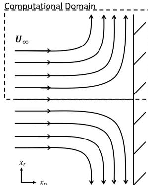
FIGURE 2. Schematic description of a flow against a vertical flat plate (Hiemenz flow). The computational domain is shown by the dashed box.
