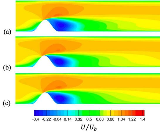
FIGURE 4. Contours of mean streamwise velocity on the bump centerplane for (a) the LES data, and the RANS momentum equations solved using filtered Reynolds stresses formed from the LES TKE and the anisotropy tensor for (b) the LES data, and (c) the three-term optimal tensor basis expansion.
