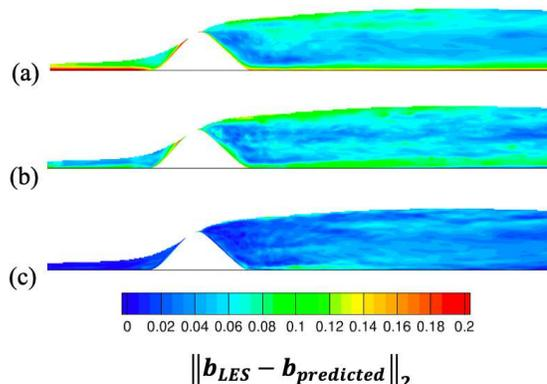
FIGURE 3. Error in the predicted anisotropy tensor with respect to LES data, measured using the 2-norm, for (a) the RKE model, (b) the three-term TBNN, and (c) the three-term optimal tensor basis expansion.
