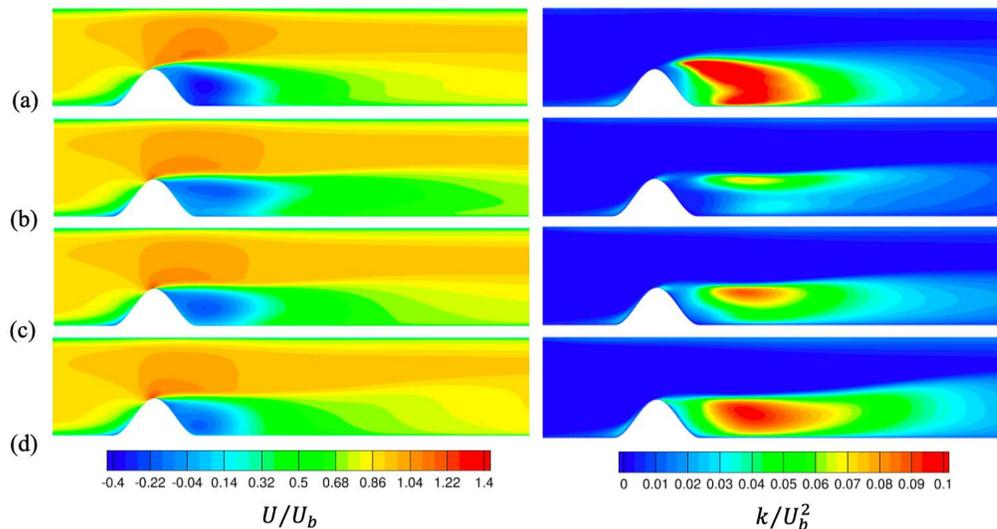
FIGURE 5. Contours of mean streamwise velocity and TKE on the bump centerplane for (a) the LES data, and the RANS momentum and auxiliary equations solved using filtered Reynolds stresses formed from the predicted TKE and the LES anisotropy tensor for (b)  $\beta = 1$ , (c)  $\beta = 0.8$ , and (d)  $\beta = 0.6$ .
