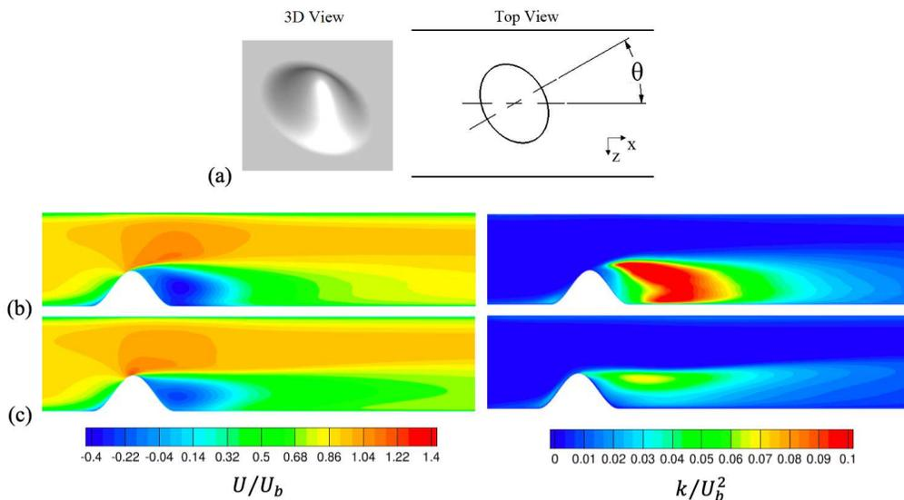
FIGURE 1. Overview of the 10 degree bump flow showing (a) isometric and top-down views of the geometry, (b) contours of LES mean streamwise velocity and turbulent kinetic energy on the bump centerplane normalized by the bulk velocity, and (c) contours of streamwise velocity and turbulent kinetic energy predicted by the RKE model on the bump centerplane.
