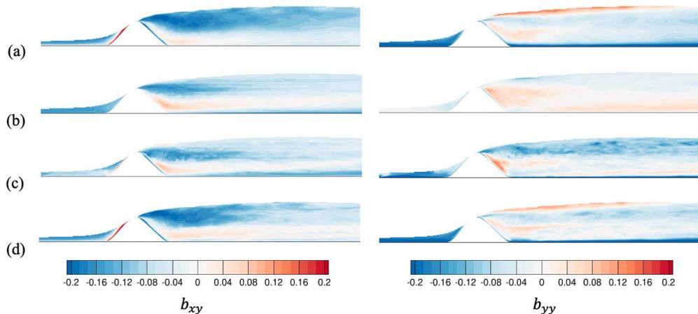
FIGURE 2. Shear stress and wall-normal (vertical) anisotropy components for (a) the LES data, (b) the RKE model, (c) the three-term TBNN, and (d) the three-term optimal tensor basis expansion.
