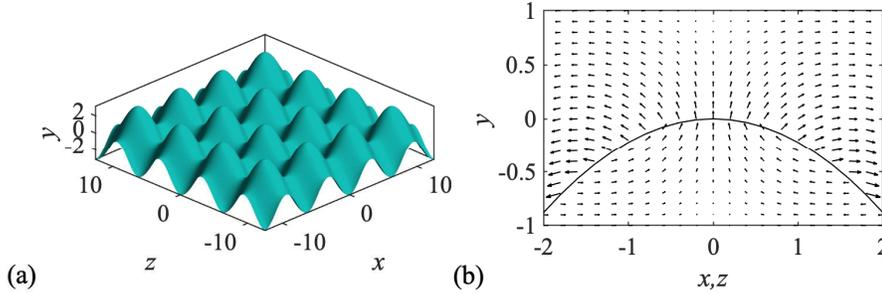
FIGURE 5. (a) Schematic view of the interface contour of 3D RTI for p4mm. (b) Qualitative velocity fields for planes at the tip of the bubble. The horizontal and vertical velocities are shown as a vector field and the interface is represented as a black solid line at  $x = 0$ ,  $y = 0$  planes.
