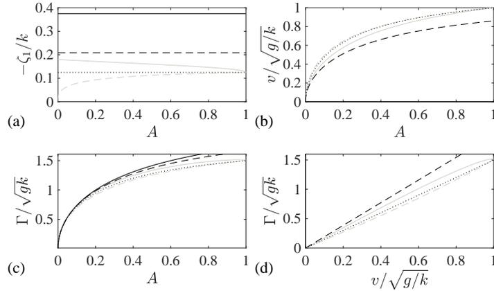
FIGURE 4. Special solutions for bubbles among the one-parameter family of asymptotic solutions with  $p4mm$ . (a) Curvature, (b) velocity and (c) shear are illustrated as a function of Atwood number  $A$ . A 1-to-1 relation between the shear and the velocity is presented in (d). Critical bubble (black solid), convergence limit bubble (black dashed), Taylor bubble (black dotted), Layzer-drag bubble (gray solid) and Atwood bubble (gray dashed).
