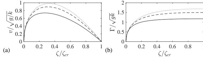
FIGURE 2. The nonlinear regime family of asymptotic solutions for the bubbles for p4mm sub-space group. The velocity  $v/\sqrt{g/k}$ , the shear  $\Gamma/\sqrt{gk}$  and the curvature  $\xi$  are shown with three different Atwood numbers,  $A = 0.3$  (solid lines),  $A = 0.6$  (dashed lines) and  $A = 0.9$  (dotted lines).
