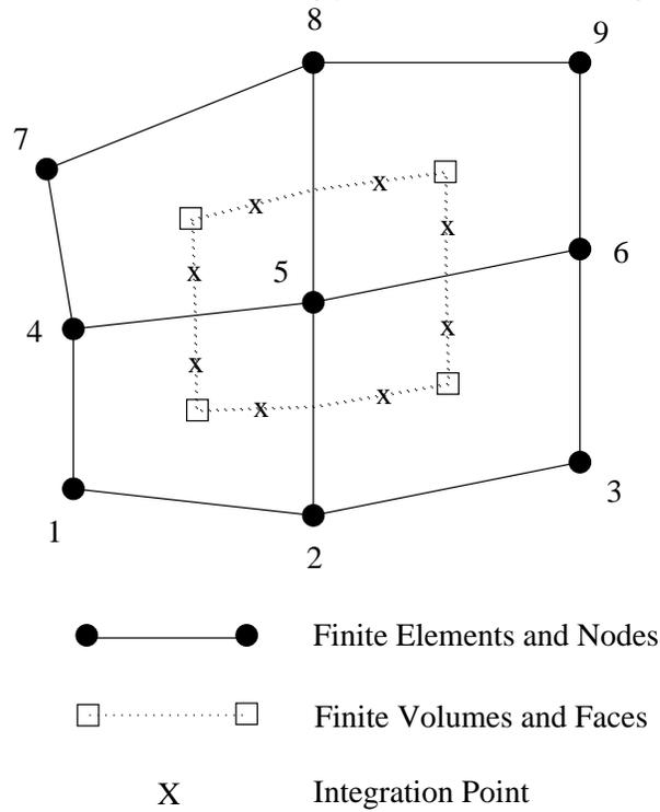
FIGURE 4. A control volume centered about a finite-element node in a collection of 2-D quadrilateral elements.
