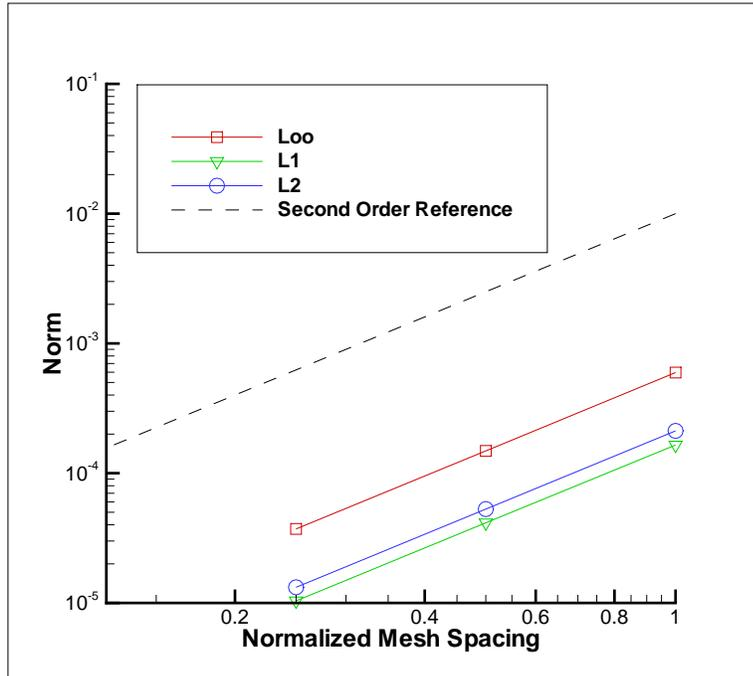
FIGURE 9. Plot of error norms vs. normalized mesh spacing for velocity using the fourth-order stabilization with characteristic scaling (variable density).
