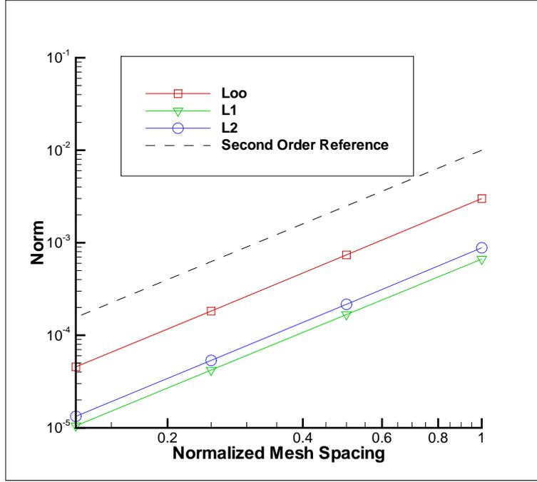
FIGURE 6. Plot of error norms vs. normalized mesh spacing for velocity using the fourth-order stabilization with characteristic scaling.
