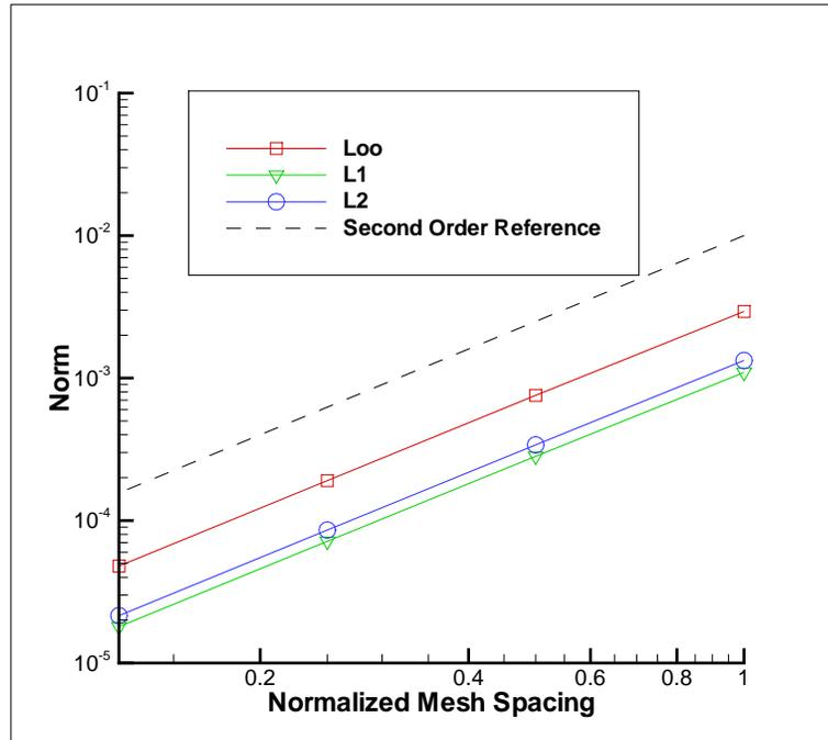
FIGURE 5. Plot of error norms vs. normalized mesh spacing for velocity using the second-order stabilization with characteristic scaling.
