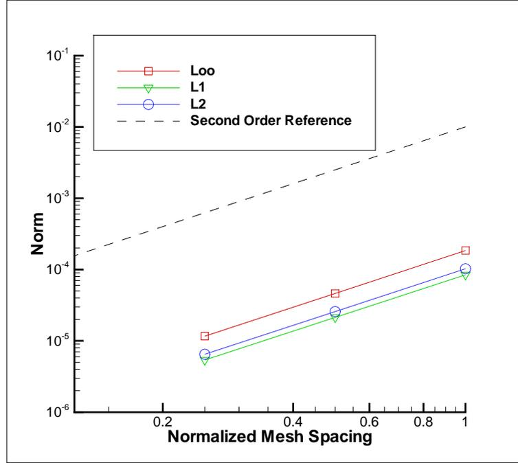
FIGURE 10. Plot of error norms vs. normalized mesh spacing for mixture fraction using the fourth-order stabilization with characteristic scaling (variable density).
