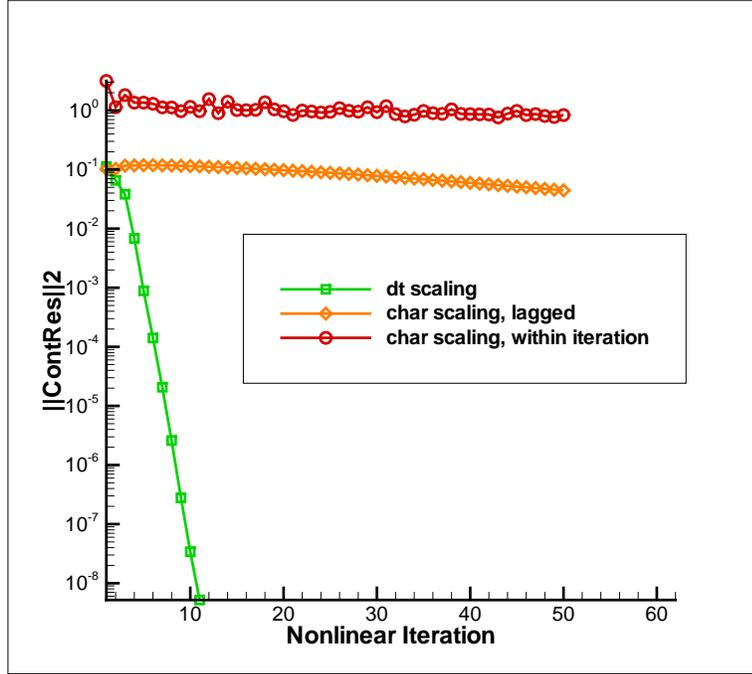
FIGURE 2. Plot of non-linear error norms within a given time step as a function of non-linear iteration comparing time step and characteristic scaling. Also shown is the effect of lagging the characteristic scaling parameter.
