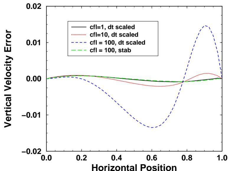
FIGURE 1. Plot of error profiles for the y-component of velocity for a driven cavity (see Ghia *et al.* 1983) flow using various time step scaling parameters. Also shown is the *stabilized* method described in Domino (2006) that uses a combination of time step and characteristic scaling.
