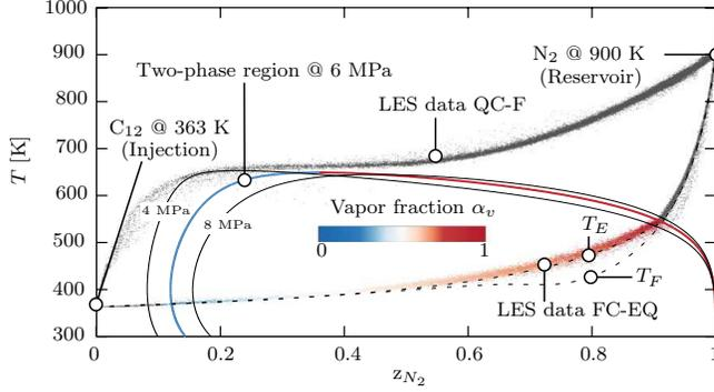
FIGURE 3. Temperature-composition diagram for a  $N_2 - C_{12}H_{26}$  mixture with frozen ( $T_F$ ) and equilibrium ( $T_E$ ) mixing temperature. Scattered data depict the thermodynamic states that are obtained in the QC-F and FC-EQ LES at  $144 \mu s$ . For FC-EQ, points within the two-phase region are colored by vapor volume fraction.
